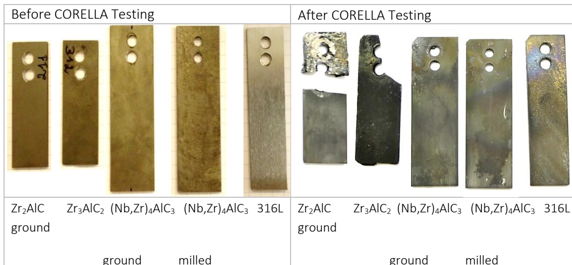
Fig. 3.2.1: Photos of specimens before and after 1000h erosion corrosion test at 500°C.
