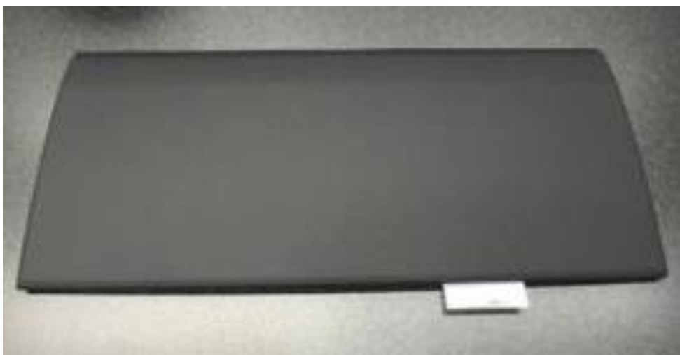
Fig. 4.4.3: Result on microwave assisted coating of Land Rover glove-box cover.
