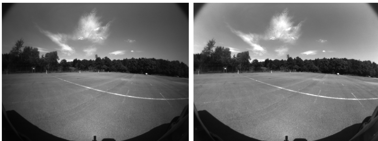
Figure 3.5: Side-by-side comparison between the original image (left) before and after applying vignetting and light falloff compensation (right). Note the severe intensity reduction towards the image boundary in the original image, and the almost even intensity across the ground in the compensated image. In the compensated image reduced brightness around the clouds in sky can be observed. This is due to overexposure in the original image.
