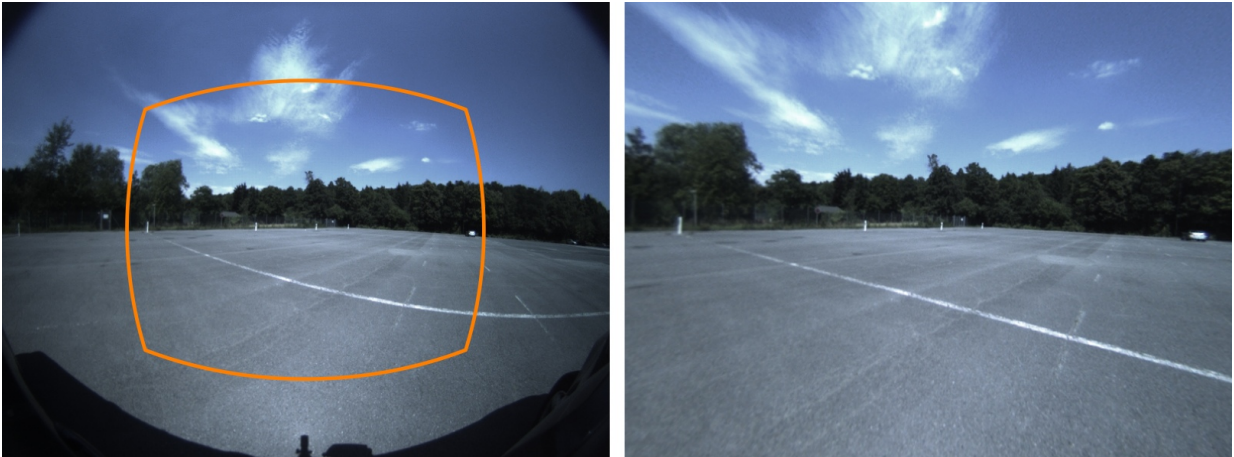
Figure 3.3: Image captured using a fisheye lens with equidistant projection (left), and corresponding image generated using a perspective camera model. The projection of the image border of the perspective image mapped into the fisheye image is shown in orange. The horizontal angle of view is 170^\circ and 100^\circ , respectively.
