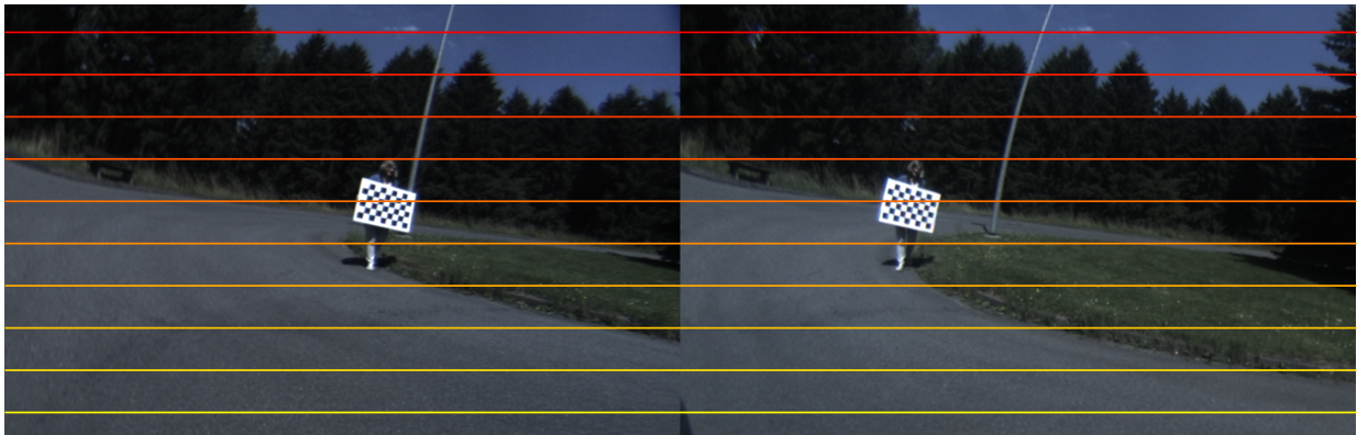
Figure 8.19: Stereo rectified image pair corresponding to Figure 8.18. For rectification the equidistant model [Abr05] was used. One can observe that, e.g. the same tiles of the calibration target are intersected by the epipolar line. The wide baseline causes the calibration target to obstruct parts of the lamp post in the left image while being considerably offset in the right image.
