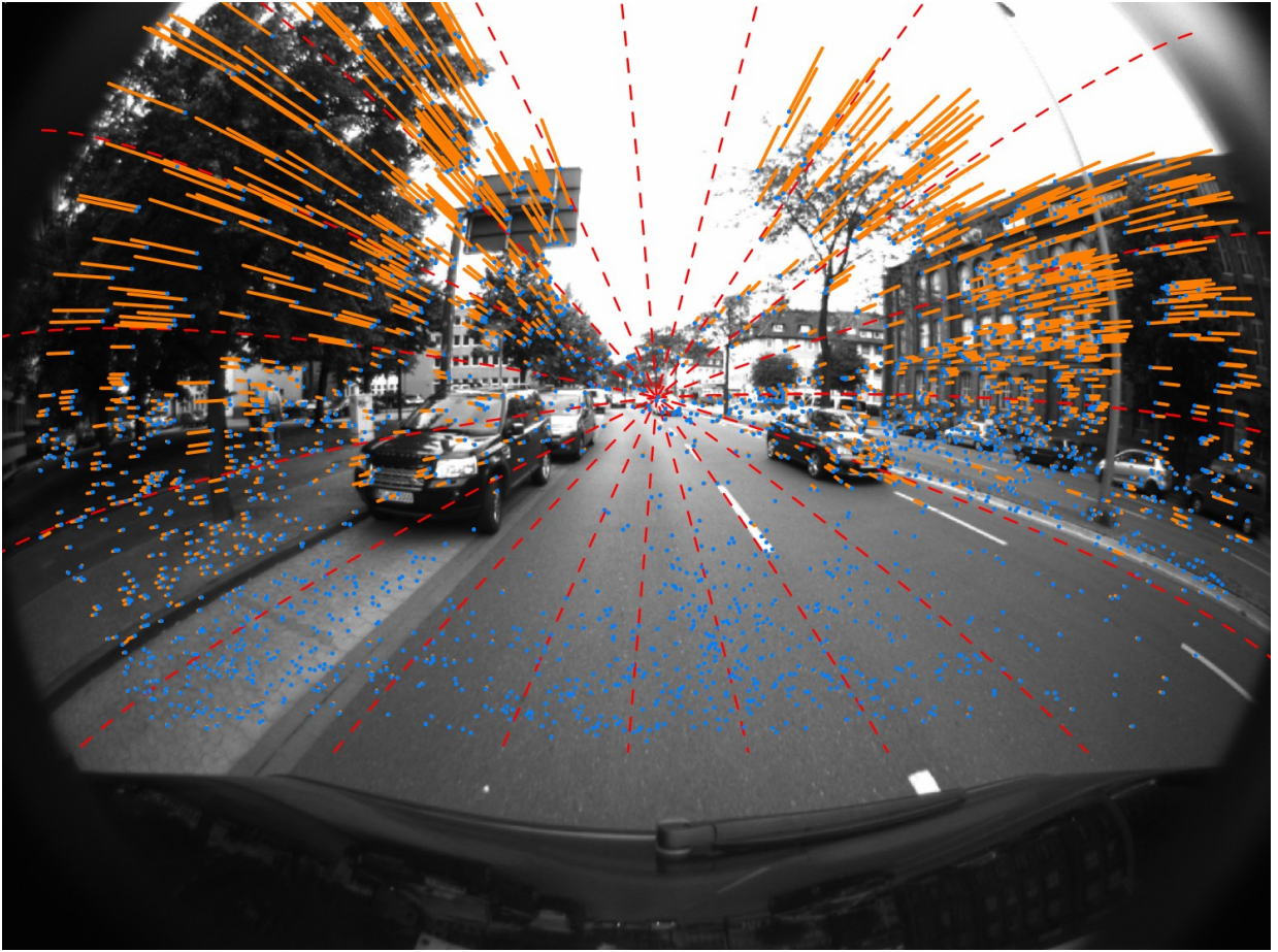
Figure 6.2: Planar parallax vectors superimposed on an image of a backward-facing camera. Feature points are shown in blue. The planar parallax with respect to the estimated ground plane is shown in orange. Notice the non-vanishing parallax on the left sidewalk. For better visualization, some feature mismatches have been removed. To visualize the epipolar field property, epipolar lines have been superimposed in red. Predicted feature positions above the horizon are caused by plane-ray intersections corresponding to antipodal rays.
