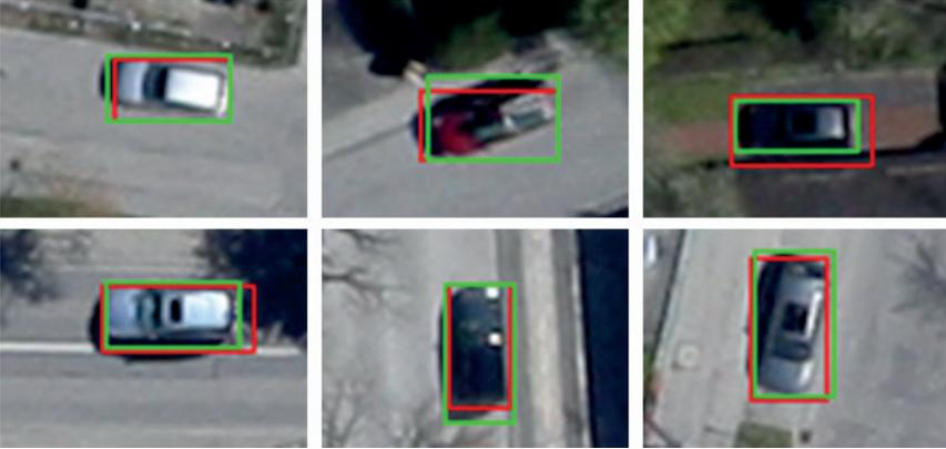
**Figure 5.4:** Qualitative detections (red boxes) and corresponding GT annotations (green boxes) for a feature map resolution of 1/4 of the input image. The detections overlap very well with the GT annotations.
