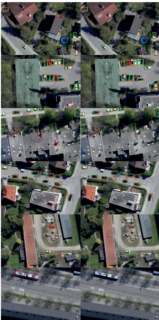
**Figure 5.8:** Qualitative detections (red boxes) and corresponding GT (green boxes) for Faster R-CNN using *conv3\_3* (left column) and our proposed DFRCNN (right column) on DLR 3K indicate that false alarms due to objects with shapes similar to vehicles are reduced by integrating more semantic information.
