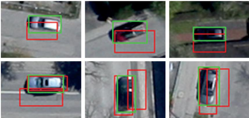
**Figure 5.3:** Qualitative detections (red boxes) and corresponding GT annotations (green boxes) for a feature map resolution of 1/16 of the input image. The detections show a relatively poor overlap with the GT annotations and multiple detections are often generated for one GT object.
