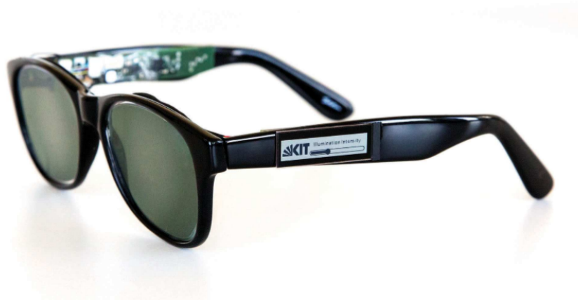
Figure 1.2: OPV integrated into sun glasses. The OPV device supplies energy for thermal and radiation intensity sensors. 6
