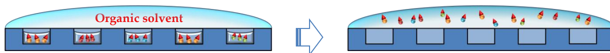
Figure 35. Removal of the polymer matrix and the excessive amino acid derivatives by dissolving them in an appropriate organic solvent. Special additives are implemented to passivate the residual monomers (the coupled amino acids are not shown for simplicity).
