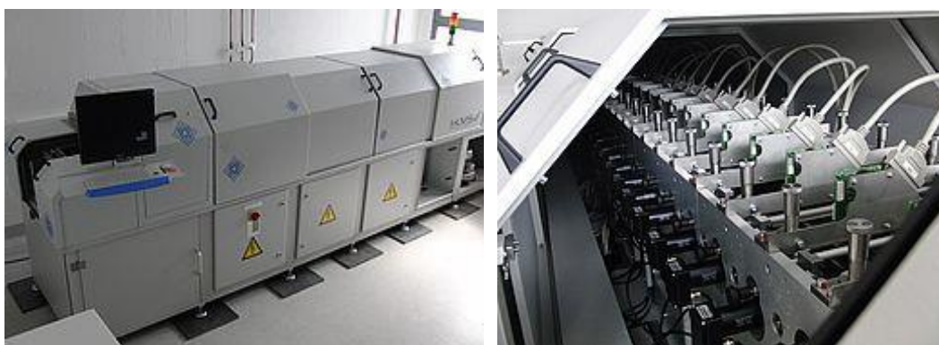
Figure 12. Peptide laser printer: (left) general view; (right) amino acid printing units (image credit: PEPperPRINT GmbH).
