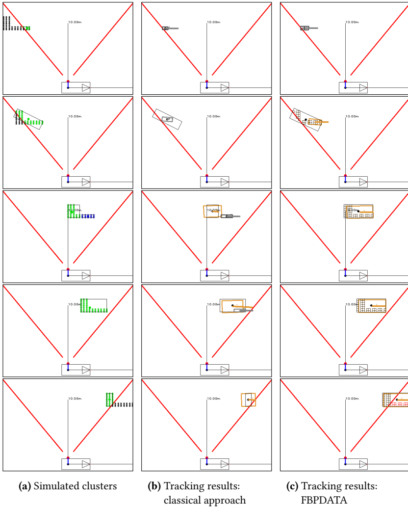
Figure 6.7: Tracking results for a simple simulated scenario with a split detection (top view; frames 2, 3, 7, 8, 10).
