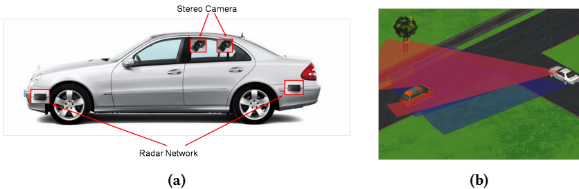
Figure 1.6: (a) Placement of the sensors in the experimental vehicle. (b) Schematic illustration of the fields of view of both sensor systems (radar: blue, video: red).
