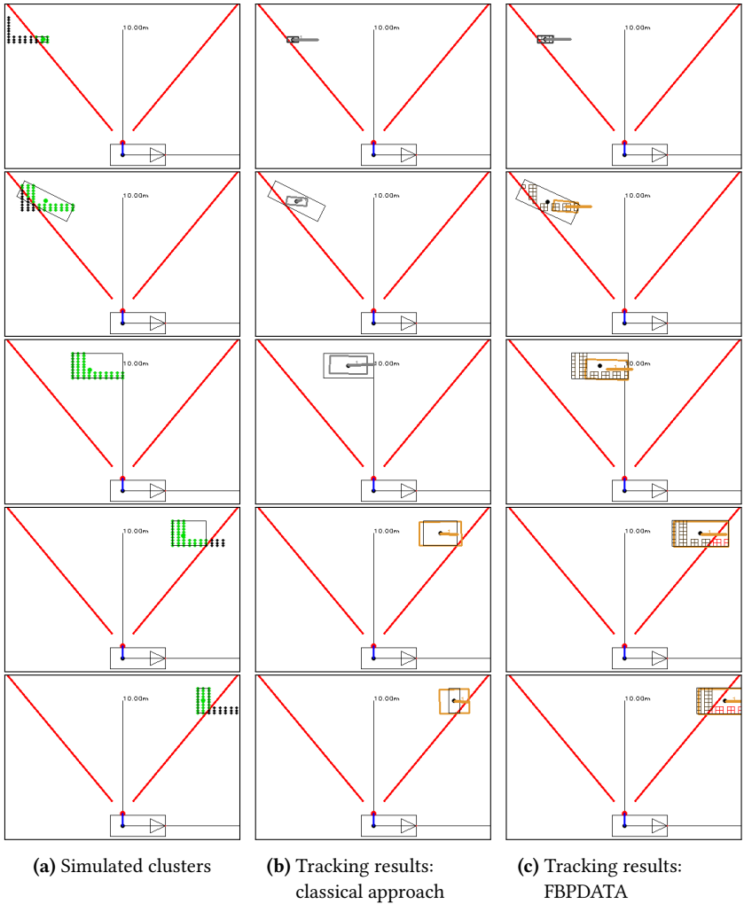
Figure 6.4: Tracking results for a simple simulated scenario with an object crossing the FoV of the sensors (top view; Frames 2, 3, 4, 8, 10).
