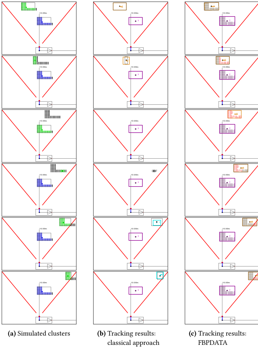
Figure 6.10: Tracking results for a simple simulated occlusion scenario (top view; frames 10, 14, 18, 20, 23, 25).
