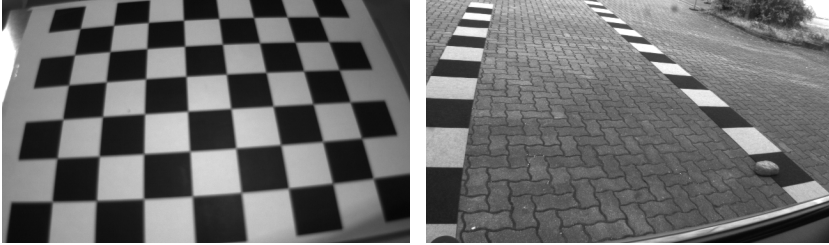
(a) Chess board pattern used for intrinsic camera calibration.
