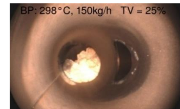
Pipe blockage by solid deposits in engine test bench (Brack 2014)
