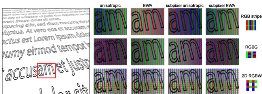
Figure 4.1: Subpixel rendering of a plane with a structured texture for different subpixel layouts, similar to those found in diverse displays nowadays. This image showcases high-quality texture filtering, one of the applications of our proposed optimal filtering framework, comparing standard filtering (anisotropic and EWA) to our subpixel-aware filtering (again, using anisotropic and EWA). Note how our method significantly reduces aliasing. Image taken from [47].
