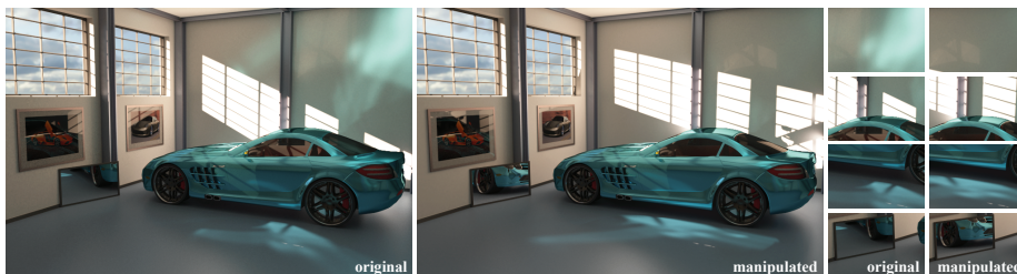
Figure 9.1: Transport manipulation in the Garage scene. Before/after close-ups (right): removing indirect highlights caused by the car, re-directing sunlight after it refracts through the windows, moving and rotating a glossy inter-reflection, and altering the mirror reflection. Image taken from [200].
