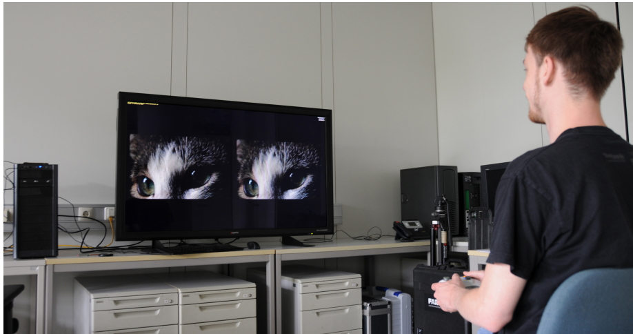
Figure 4.10: Test setup for the user study. Lighting conditions in the photograph do not match actual testing conditions, where the environment illumination was completely darkened. Image taken from [47].
