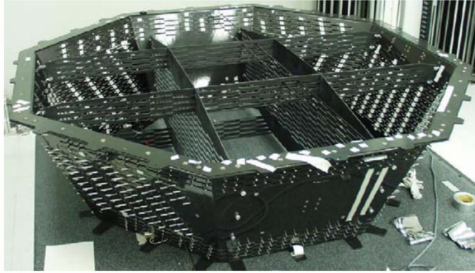
Figure 2.2.: Aluminum honeycomb support structure of the TRD allowing for a high acceptance space qualified detector with a weight of less than 500 kg [111].
