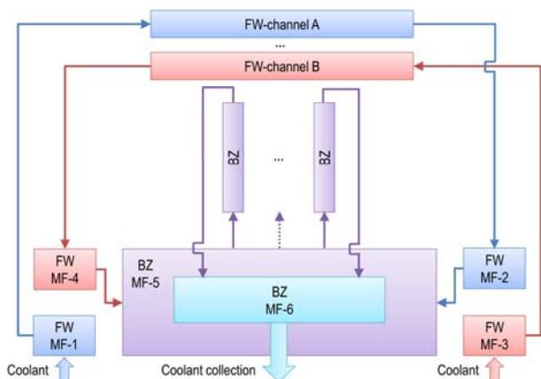
Fig. 2 Schematic flow scheme of the current MLCB
