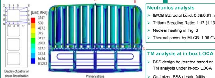
Fig. 5 Primary stress under in-box LOCA
