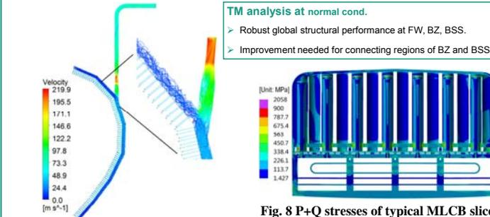
Fig. 7 Streamline at inboard BZ outlet manifold
