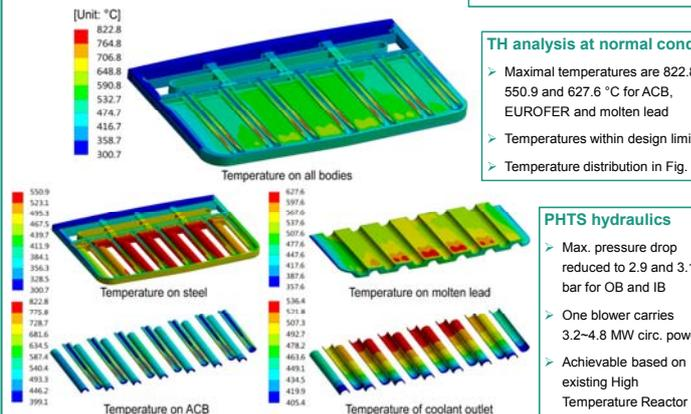
Fig. 6 Temperature distribution of typical MLCB unit slice
