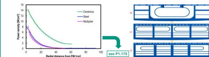
Fig. 3 Power densities of different materials
