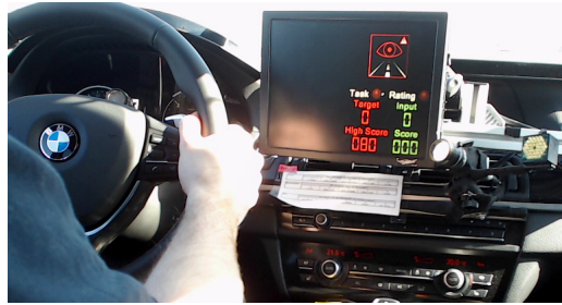
Figure 6.6: Visually demanding secondary task and the visual component of the distraction warning. The secondary task required reading random numbers 1 and 2 shown in green in the right lower quarter of the display. The visual component of the warning consisted of a red warning icon shown in the right upper corner of the display.
