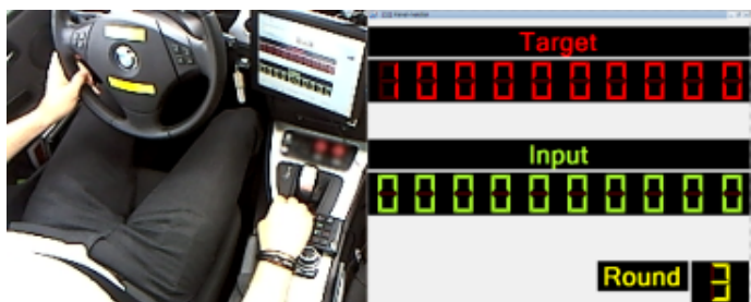
Figure 4.9: Artificial secondary task used in the first driving experiment. Left picture shows the vehicle’s interior, where the driver is reading the random numbers from the display and typing by means of a number pad. The right picture shows the presentation of the random numbers.
