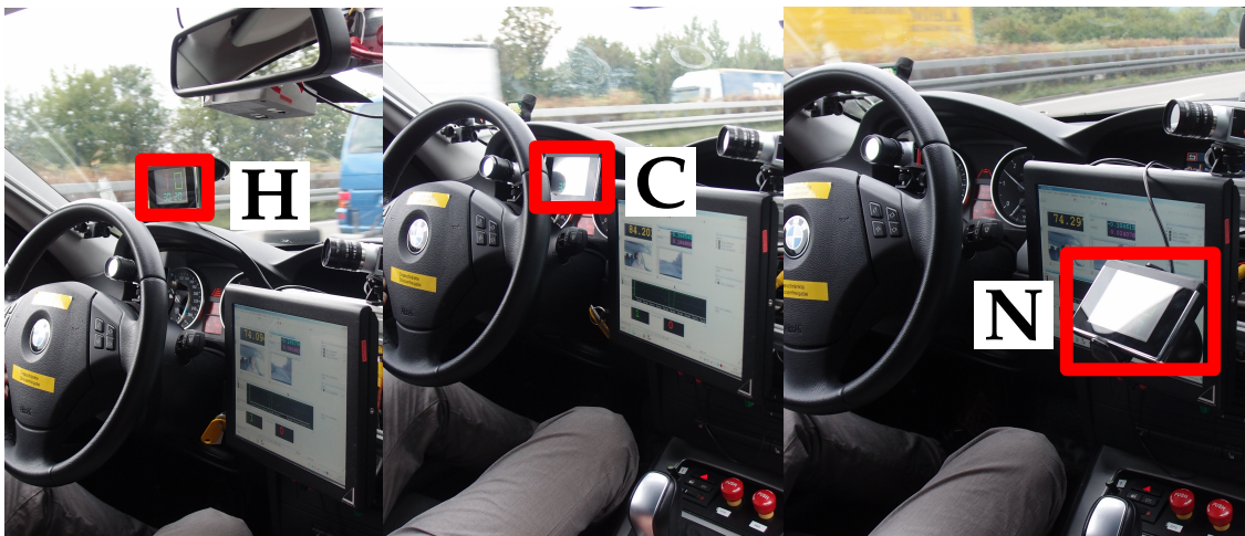
Figure 5.4: The positions of the display used in the experiment. H is a display position that requires an amount of gaze aversion similar to a Head-Up display, C is the position of the vehicle's r.p.m. counter and N corresponds to the vehicle's built in display for navigation.
