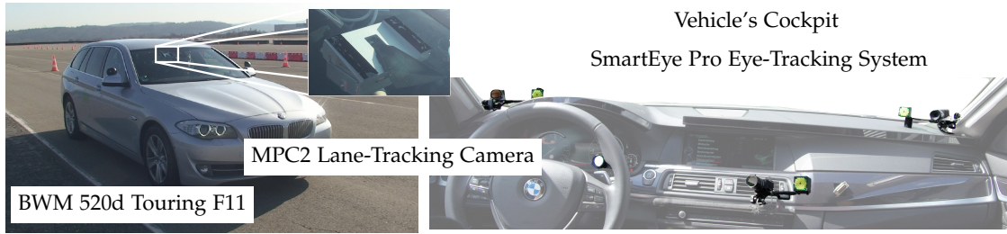
Figure 6.2: Test vehicle in user test. Left picture shows the vehicle and the MPC2 camera, right picture shows the individual cameras of the eye-tracking system in the vehicle's cockpit.
