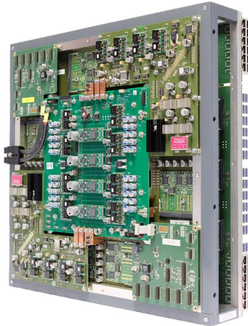
Figure 2.11: A photograph of a single fully assembled wafer module [80, 95].
