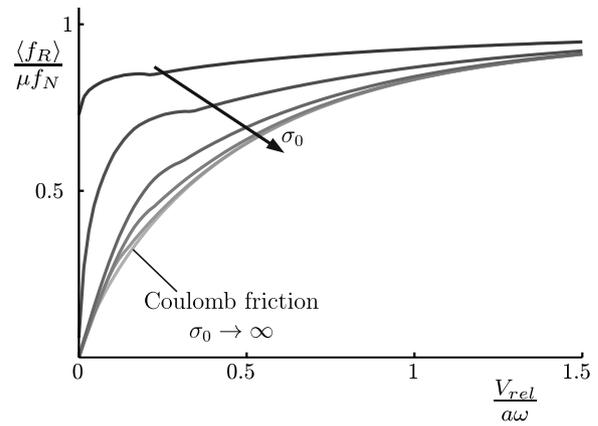
Figure 2: Effective friction-velocity characteristics for transverse excitation
