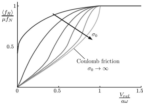
Figure 1: Effective friction-velocity characteristics for longitudinal excitation
