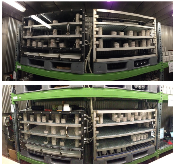
Figure A.1: Boxes for storing of the concrete samples at ambient temperature
