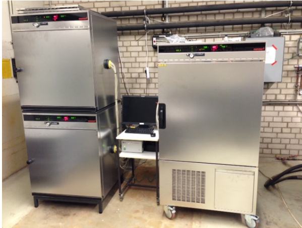
Figure A.2: Climate chambers for storing the concrete samples at elevated temperatures
