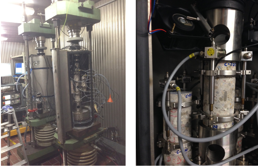
Figure A.5: Preparation of the samples shortly before conducting creep tests at elevated temperatures. Creep climate chambers integrated to the testing machines (left) and detailed view of the samples equipped with inductive displacement transducers (right)
