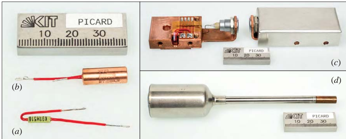
Figure 3.4: Pictures of TVO temperature sensors installed in PICARD: (a) plain TVO, (b) TVO cast in a copper cartridge, (c) cast TVO inserted into a copper block with aluminium radiation shield for surface temperature measurement, and (d) cast TVO at the tip of a thermally insulated stick for in-tube temperature measurement [26].
