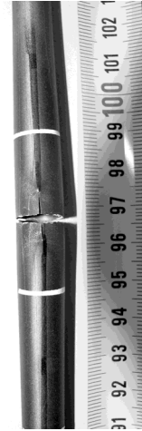
rod #13: rupture at burst middle
