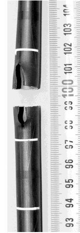
rod #14: rupture at burst middle
