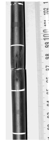
rod #21: rupture at burst middle
