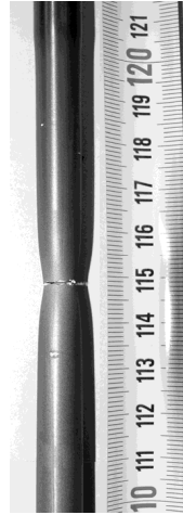
rod #11: rupture at upper sample holder
