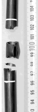
rod #2: 2 ruptures along hydrogenated bands
