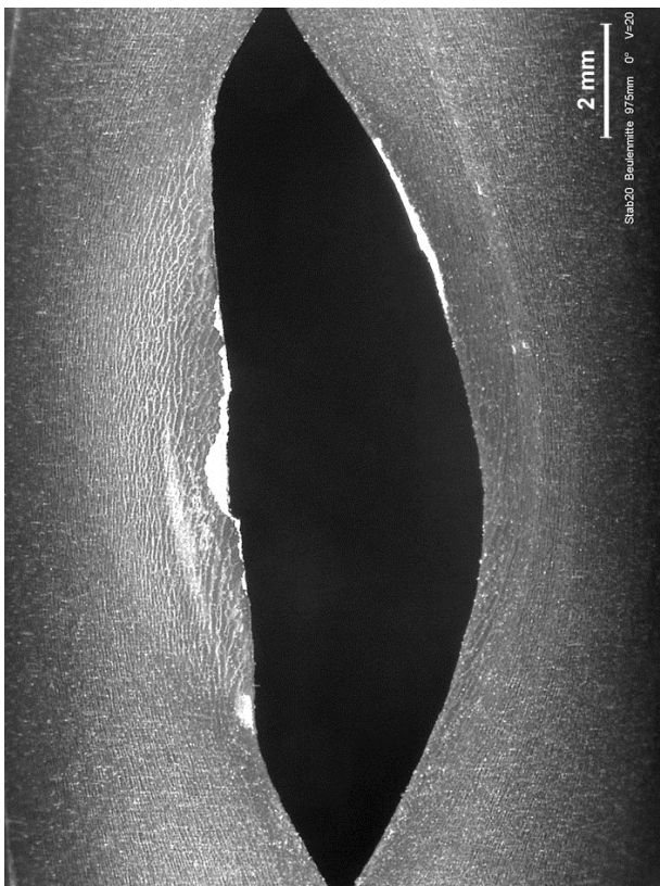
Rod #20 at 325°; p=50 bar, A_{burst}=53 \text{ mm}^2
