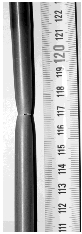
rod #16: rupture at upper sample holder
