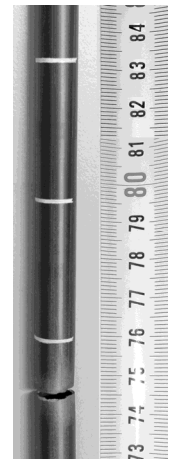
rod #17: rupture at stuck pellet
