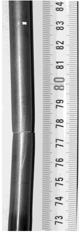
rod #10: rupture at low sample holder
