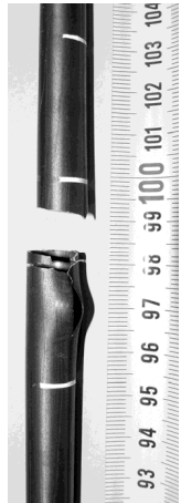
rod #5: rupture and crack at upper hydrogenated band
