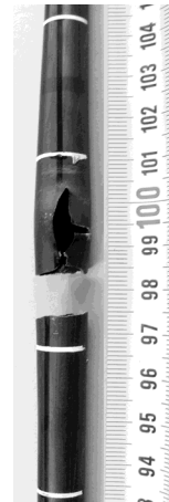
rod #7: middle cross crack and rupture at low hydrogenated band
