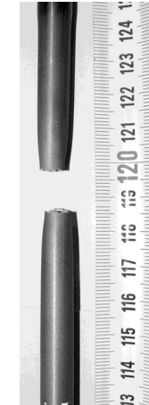
rod #9: rupture at upper rod holder
