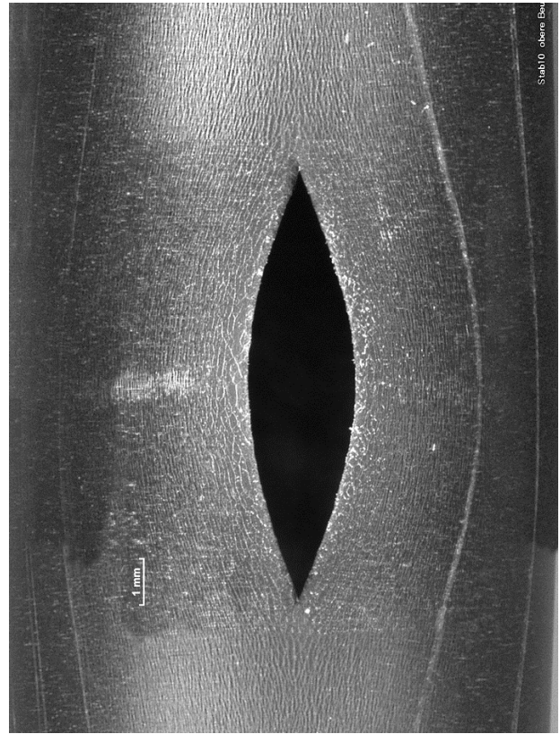
Rod #10 at 77°; p=45 bar, A_{burst}=13 \text{ mm}^2
