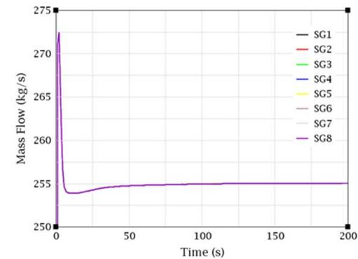
**TRACE: Convergence behaviour of mass flow rate through all SGs (8)**
