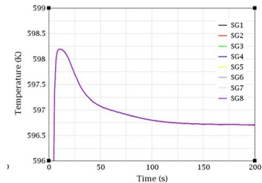
**TRACE: Convergence behaviour of the Coolant temperature at the SG-inlet**
