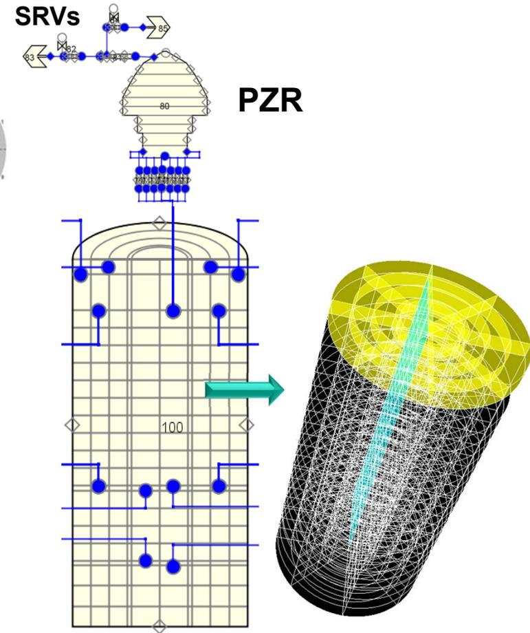
3D VESSEL Cylindrical Model (21x5x8 cells)
