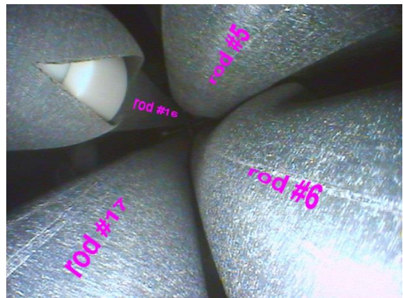
at corn. rod B, elevation 950 mm: fragmented pellets blocked the burst opening of rod #16
