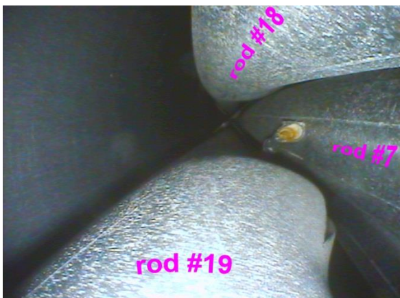
at corn. rod C, elevation 950 mm: TC TFS 7/13, bending of rod #18
