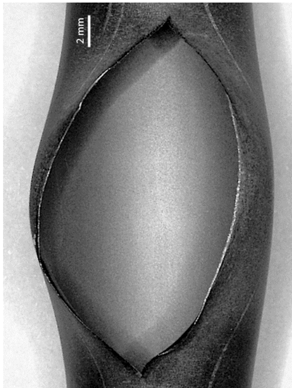
Rod #5 at 270°, A_{burst} = 198 \text{ mm}^2
