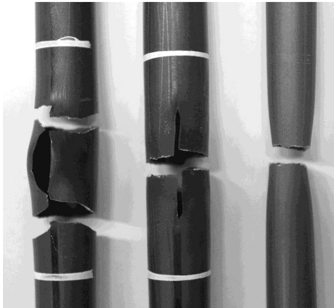
hydrogen embrittlement (inner rods with C_H \sim 2000 wppm) stress concentration (outer rods with C_H \sim 1000 wppm) necking (outer rods)
