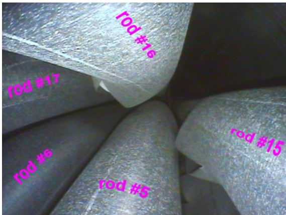
at corn. rod B, elevation 950 mm: bending of rod #17
