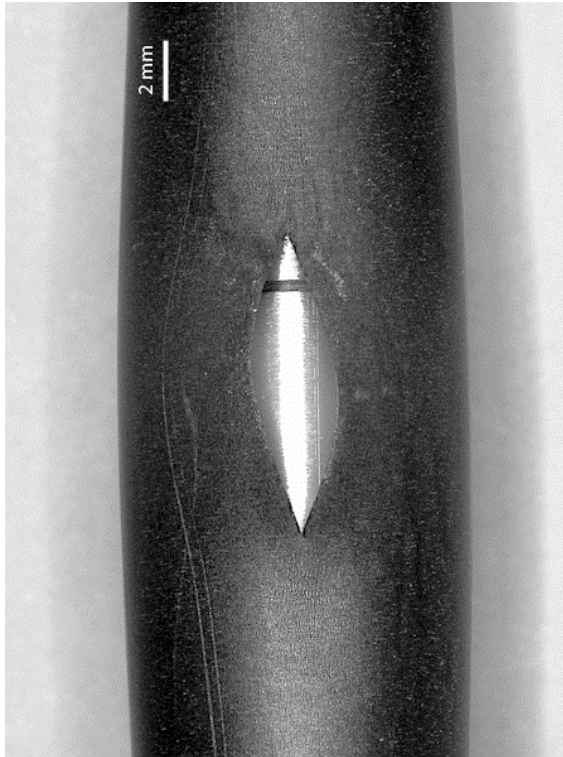
Rod #18 at 45°, A_{burst} = 17 \text{ mm}^2
