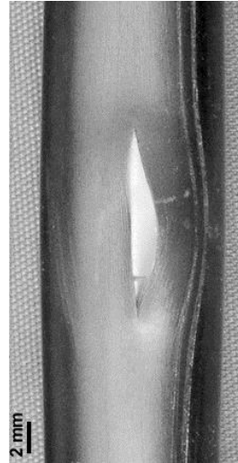
rod #8 at 100°, A_{burst} = 24 \text{ mm}^2 , w_{burst} = 3.3 \text{ mm}
