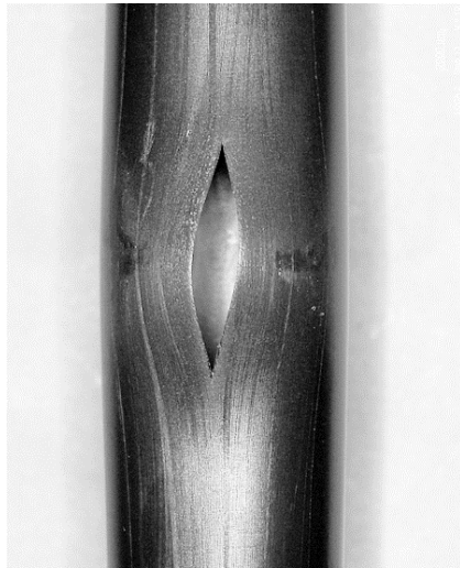
rod #13 at 151°, A_{burst} = 15 \text{ mm}^2 , w_{burst} = 2.4 \text{ mm}
