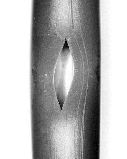
rod #18 at 274°, A_{burst} = 24 \text{ mm}^2 , w_{burst} = 3.3 \text{ mm}
