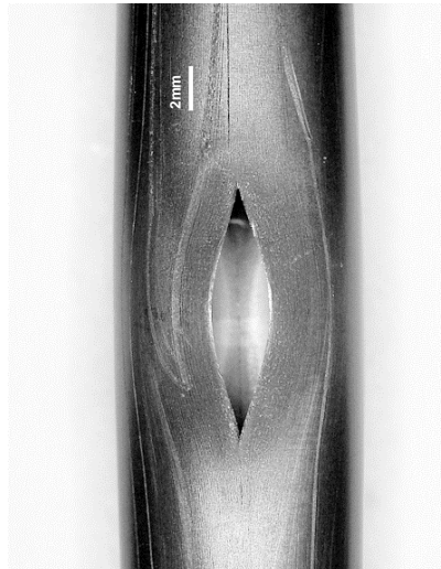
rod #14 at 129°, A_{burst} = 23 \text{ mm}^2 , w_{burst} = 3.1 \text{ mm}
