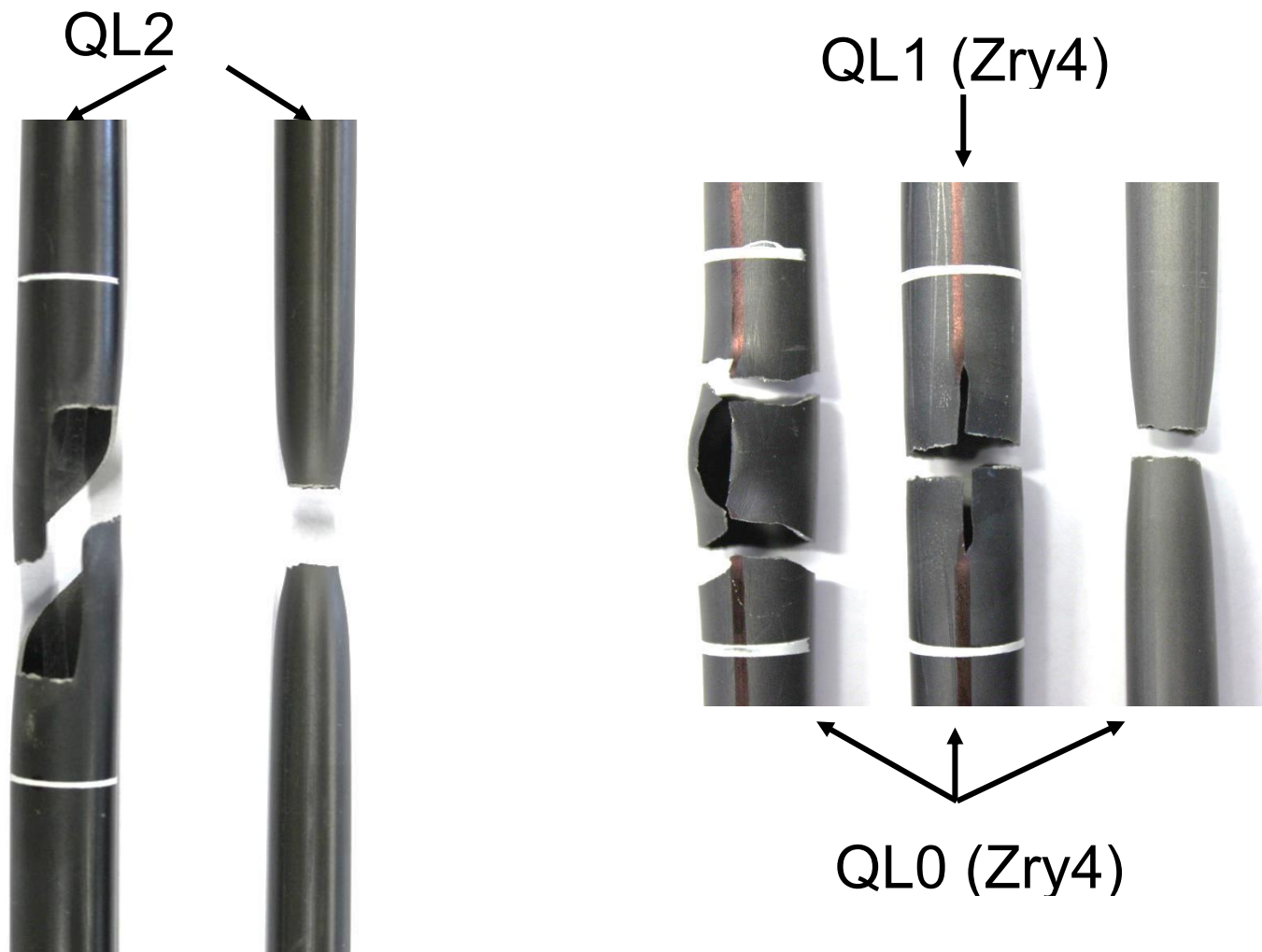
Figure 115 Failure modes of post tensile tested QUENCH-LOCA claddings; left: M5 ® (QUENCH-L2) and right: Zircaloy-4 (QUENCH-L0 and QUENCH-L1).
