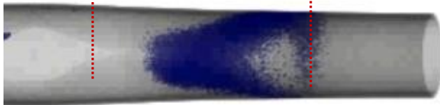
neutron tomography above burst opening: localization of hydrided region (blue)
