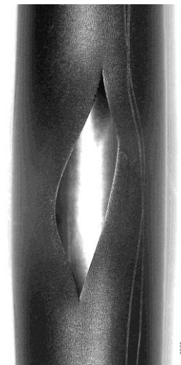
#21 at 5°, A_{burst} = 40 \text{ mm}^2 , w = 4.1 \text{ mm} ; h = 17.5 \text{ mm}
