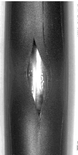
#17 at 260°, A_{burst} = 28 \text{ mm}^2 , w = 3.6 \text{ mm} , h = 14 \text{ mm}
