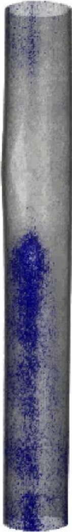
rod #13: hydrogen spot eventually at contact pellet-cladding
