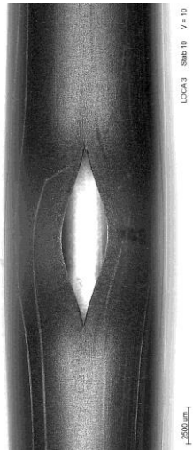
#10 at 36°, A_{burst} = 24 \text{ mm}^2 , w = 3.4 \text{ mm} , h = 13 \text{ mm}
