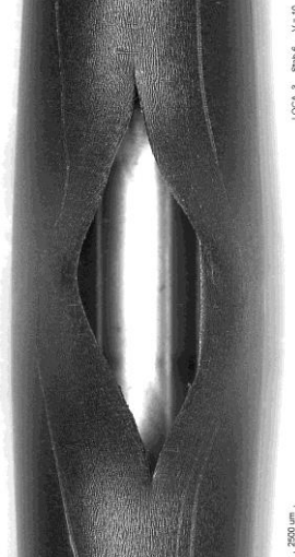
#6 at 186°, A_{burst} = 67 \text{ mm}^2 , w = 6.2 \text{ mm} ; h = 20 \text{ mm}
