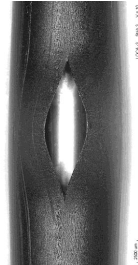
#3 at 205°, A_{burst} = 37 \text{ mm}^2 , w = 4.6 \text{ mm} , h = 15 \text{ mm}
