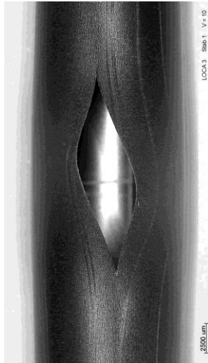
#1 at 191°, A_{burst} = 36 \text{ mm}^2 , w = 4.7 \text{ mm} , h = 16 \text{ mm}
