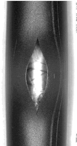
#11 at 122°, A_{burst} = 33 \text{ mm}^2 , w = 4.1 \text{ mm} , h = 14.5 \text{ mm}
