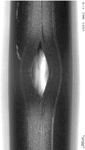
#2 at 77°, A_{burst} = 21 \text{ mm}^2 , w = 3.2 \text{ mm} , h = 11.5 \text{ mm}
