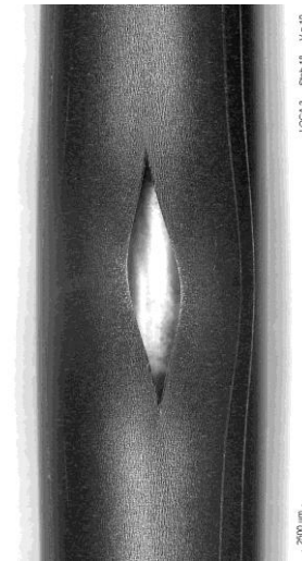
#18 at 290°, A_{burst} = 17 \text{ mm}^2 , w = 2.6 \text{ mm} ; h = 12.5 \text{ mm}
