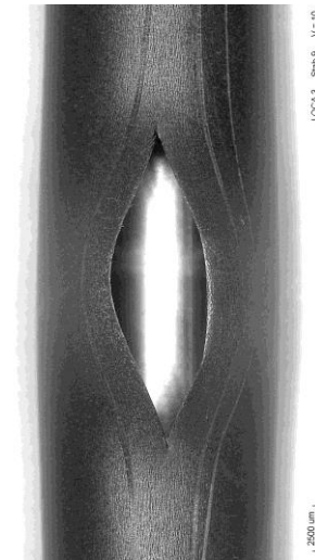
#9 at 15°, A_{burst} = 43 \text{ mm}^2 , w = 4.7 \text{ mm} , h = 16 \text{ mm}
