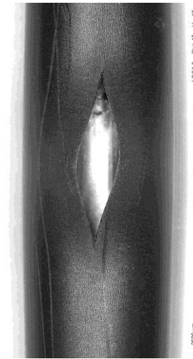
#15 at 232°, A_{burst} = 24 \text{ mm}^2 , w = 3.3 \text{ mm} , h = 13.5 \text{ mm}
