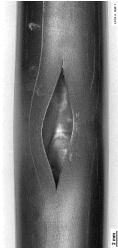
rod #7: burst at 210°; A_{burst}=33.6 \text{ mm}^2 , w=4.0 \text{ mm} , h=15.6 \text{ mm}
