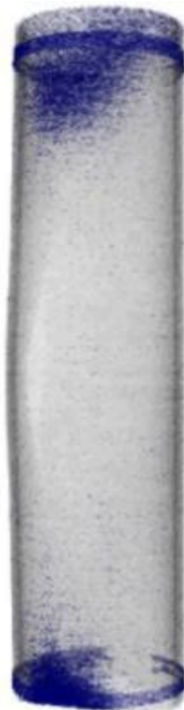
rod #9; H-band (sample top): 1490 wppm; H-spot (sample bottom): 1740 wppm
