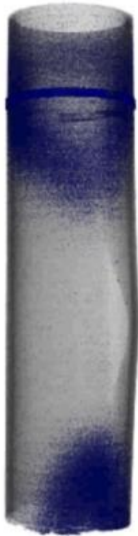
rod #1; H-band (sample top): 1720 wppm, H-spot (sample bottom): 1740 wppm
