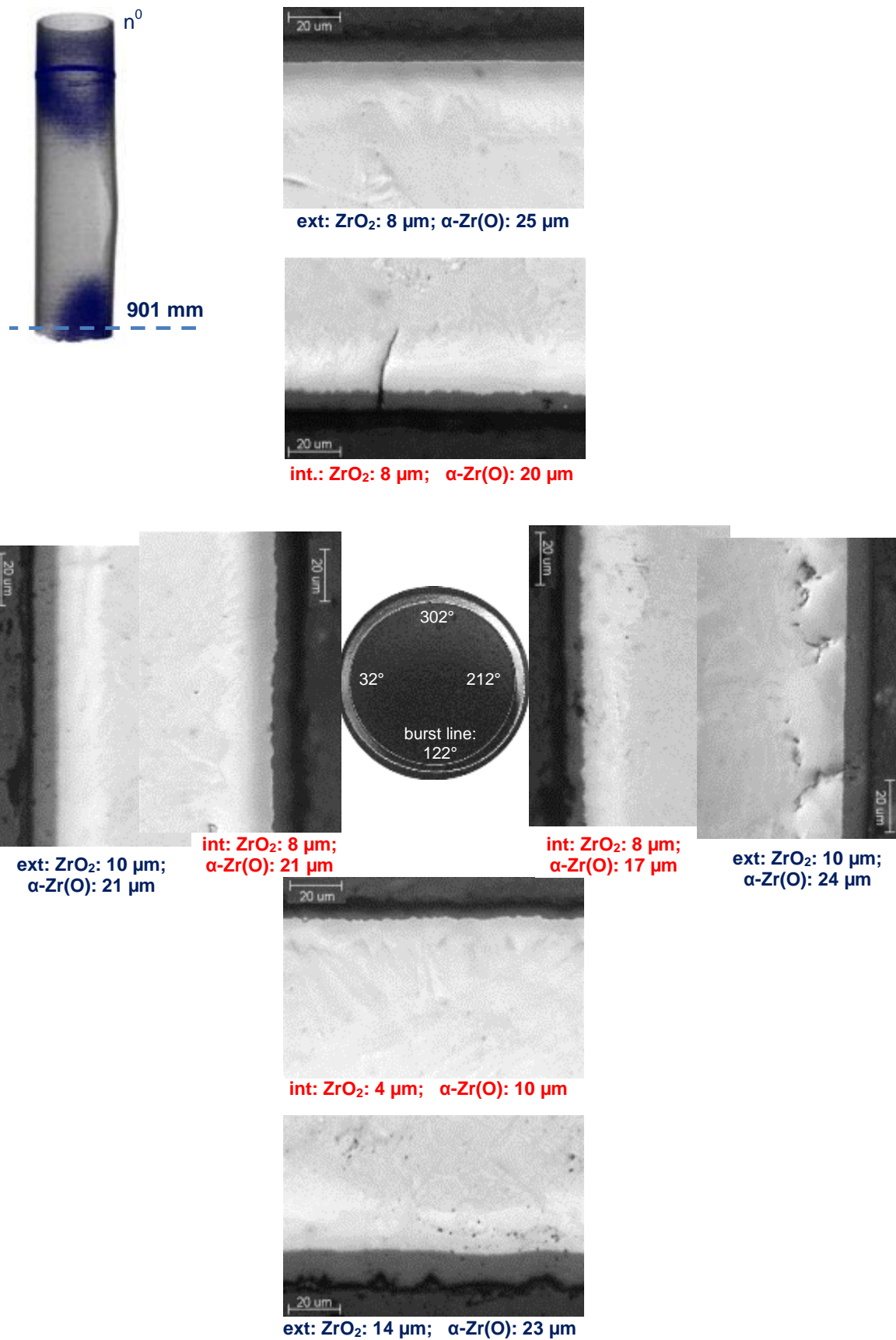
Figure 143 QUENCH-L4; Thicknesses of ZrO_2 and \alpha -Zr(O) layers at outer and inner surfaces of cladding #1 underneath burst at bundle elevation 901 mm; top view, as polished.
