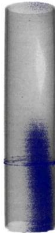
rod #6; H-spot (sample bottom): 1750 wppm
