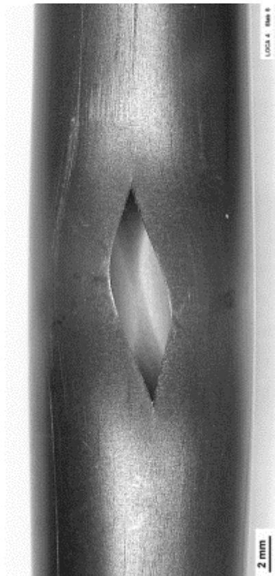
rod #8: burst at 156°; A_{burst}=21.4 \text{ mm}^2 , w=3.2 \text{ mm} , h=11.8 \text{ mm}
