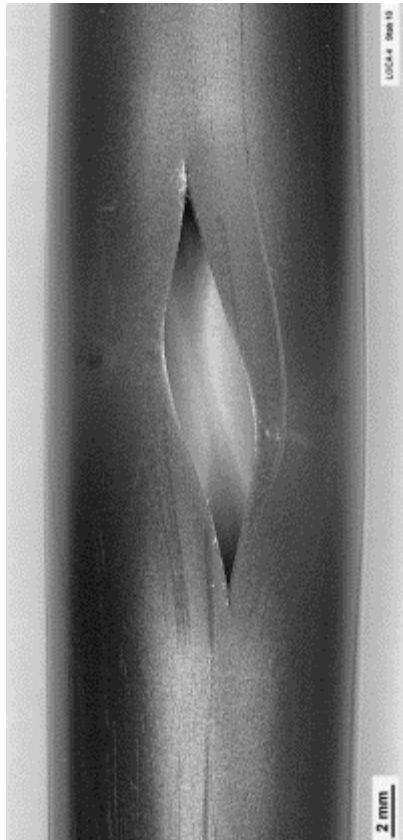
rod #10: burst at 90°; A_{burst}=25.6 \text{ mm}^2 , w=3.4 \text{ mm} , h=15.8 \text{ mm}
