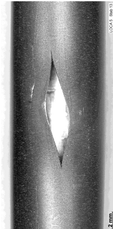
rod #13: burst at 180°; A_{burst}=19 \text{ mm}^2 , w=2.7 \text{ mm} , h=13 \text{ mm}
