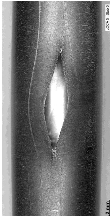
rod #5: burst at 203°; Aburst=21 mm 2 , w=3.0 mm, h=13 mm
