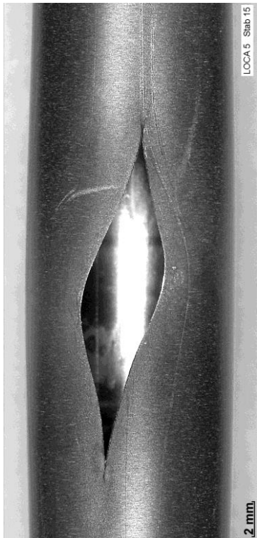
rod #15: burst at 182°; A_{burst}=40 \text{ mm}^2 , w=4.6 \text{ mm} , h=18 \text{ mm}
