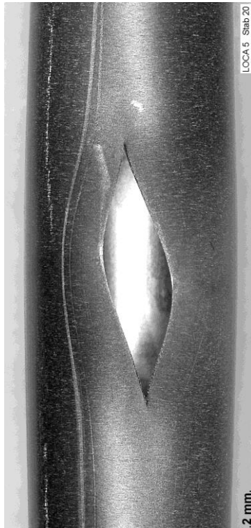
rod #20: burst at 99°; A_{burst}=29 \text{ mm}^2 , w=3.6 \text{ mm} , h=14 \text{ mm}
