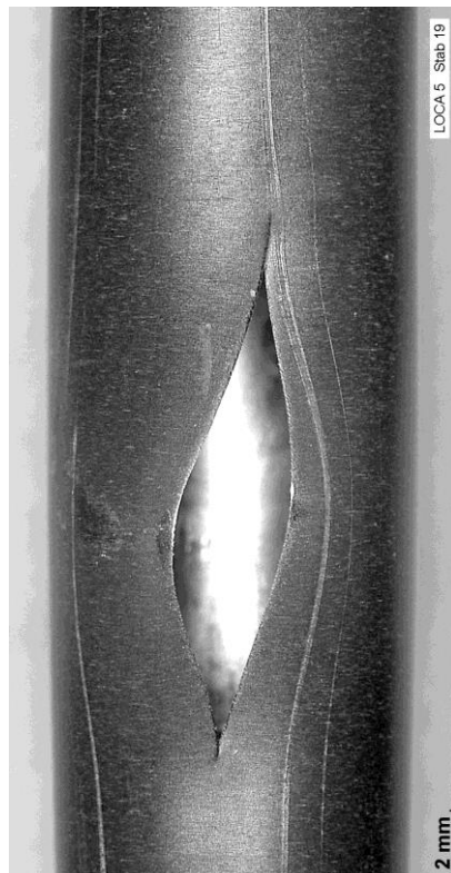
rod #19: burst at 280°; Aburst=29 mm 2 , w=3.5 mm, h=14.5 mm
