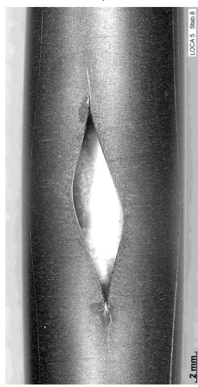
rod #8: burst at 147°; Aburst=21 mm 2 , w=3.2 mm, h=13 mm
