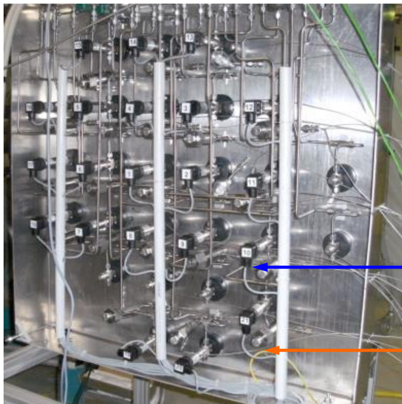
Figure 19 QUENCH-L5; Rod pressure control and measurement panel.
