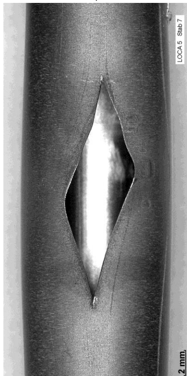
rod #7: burst at 196°; Aburst=46 mm 2 , w=4.9 mm, h=17.5 mm
