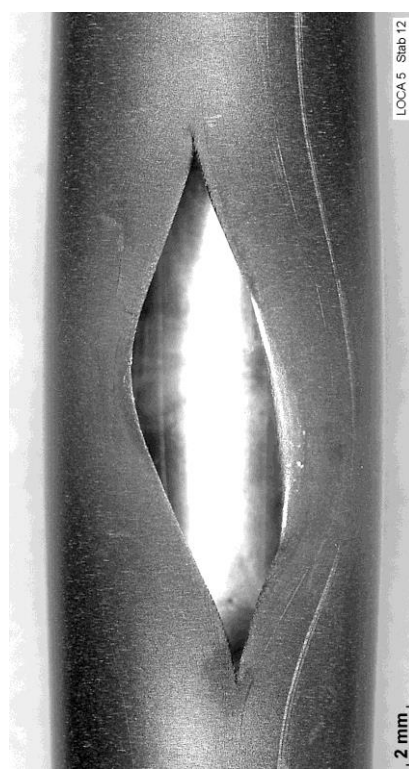
rod #12: burst at 175°; A_{burst}=52 \text{ mm}^2 , w=4.9 \text{ mm} , h=18 \text{ mm}
