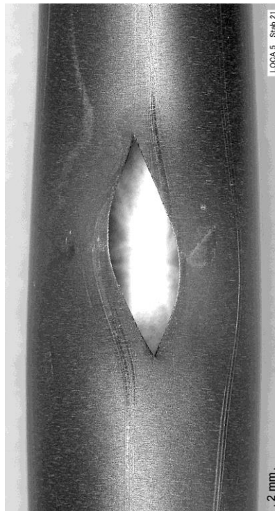
rod #21: burst at 317°; A_{burst}=28 \text{ mm}^2 , w=3.8 \text{ mm} , h=12 \text{ mm}
