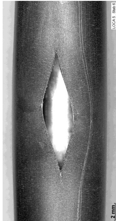
rod #6: burst at 232°; Aburst=27 mm 2 , w=3.6 mm, h=14 mm
