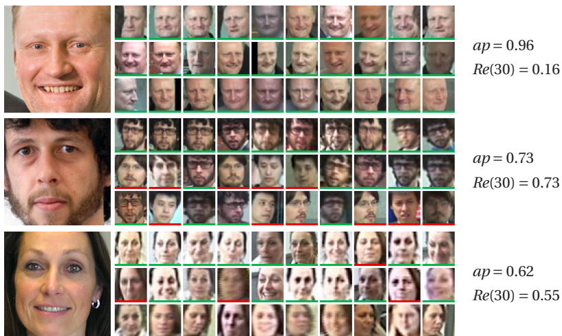
Figure 6.12: Top 30 search results for querying with the high-quality mugshot-like face images depicted on the left. Correct matches are indicated in green and average precision and recall are denoted for each query individually.
