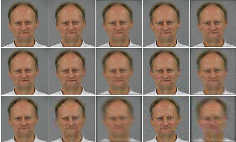
Figure 2.2: Illustration of the amplification effect of low resolution on further effects. From left to right: none, compression artifacts, motion blur, Gaussian noise and a combination of all. Face width decreases from top to bottom: 128, 64 and 32 pixels.
