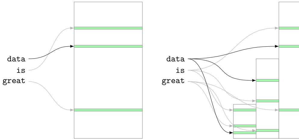
Figure 3.7: Access pattern for indices with one and three subindices and a single hash function.
