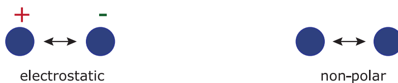
Figure 2.1: The main bonded and non-bonded interactions of atoms in the force field description. Bonded interactions consist of stretching of bonds, opening/closing of angles and out of plane rotation of bonds. Non-bonded interactions are Coulomb electrostatics and non-polar (van der Waals) interactions described as Lennard-Jones interactions.
