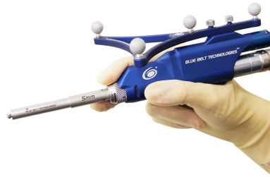
(b) Handheld semi-active robot with 1-DoF, Navio precision freehand sculptor [18] 8
