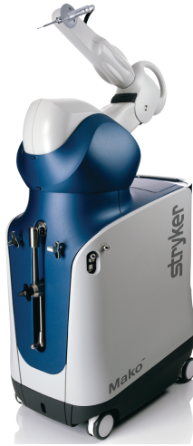
(a) Haptic semi-active robot with 6-DoF, RIO [39] 7
