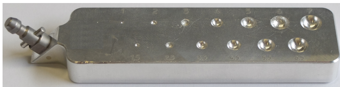
(a) Pivoting calibration plate with different molds
