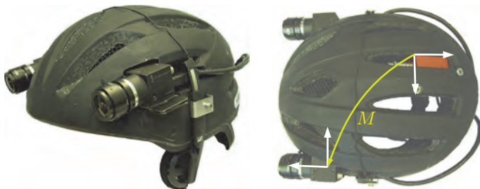
Figure 4.1: Experimental setup used to record data from an egocentric viewpoint. It is equipped with cameras, an IMU (orange) and attached headphones.
