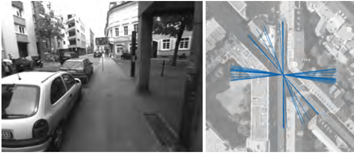
Figure 3.3: Vanishing directions detected independently from 10 slightly different viewpoints in a sequence of images. Most detections are correct in terms of the scene layout, but show varying amounts of noise. Background image: Google Earth, © 2009 GeoBasis-DE/BKG.
