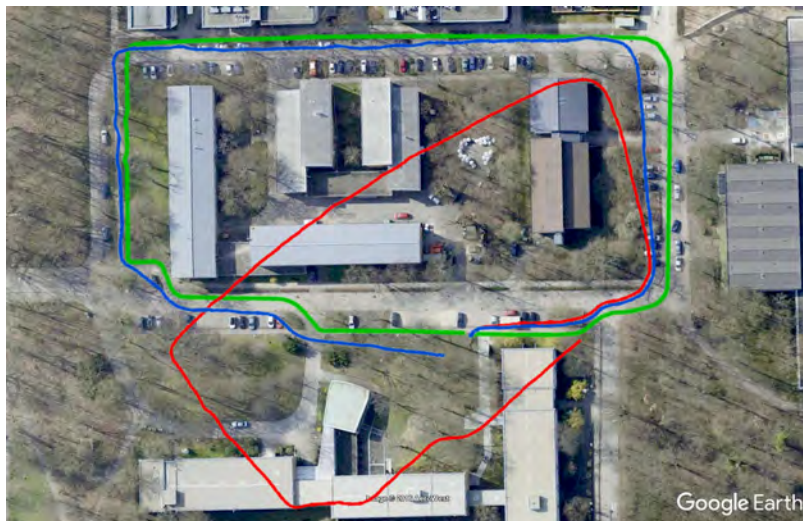
Figure 2.4: Odometric position estimation is afflicted with drift. The red path is a visual odometry estimate of the true path indicated in green. The sequence is captured with a head-worn binocular camera during walking. The cameras are subject to strong egomotion which leads to increased inaccuracies when compared to e.g. wheeled platforms. A visual inertial filter can compensate for the drift by incorporating the referenced heading and tilt measurements of an inertial measurement unit (blue path) [100]. Background image: Google Earth, © 2016 AeroWest.
