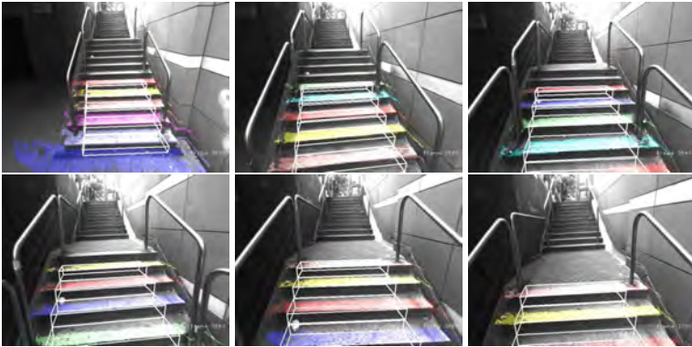
Figure 3.29: Tracking of a staircase: Visible step tracks are overlaid with different colors to indicate their identity. Cubes visualize position and size of measured steps.
