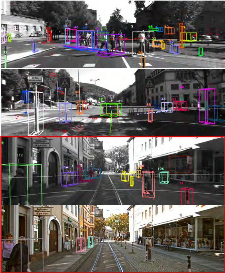
Figure 3.46: Some example scenes from a binocular camera in an automotive setup (part of the Kitti benchmark suite [27]). The perception range was increased to 30 m here. Besides traffic participants like cars, cyclists and pedestrians, also small obstacles like poles, bushes and signposts are recognized. The last two pictures show a comparison to related work of [68], in which semantic labels are used to filter objects from background.
