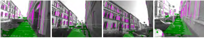
Figure 3.22: Sequence with ground plane not in free view due to camera inclination (third image). Only the vanishing direction is considered here to correct the plane parameters.
