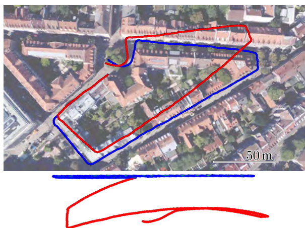
Figure 3.37: Comparison of filtered trajectory (blue) and plain visual odometry (red) in an outdoor scenario. Only the vertical vanishing direction was used to correct the odometry. Background image: Google Earth, © 2009 GeoBasis-DE/BKG.
