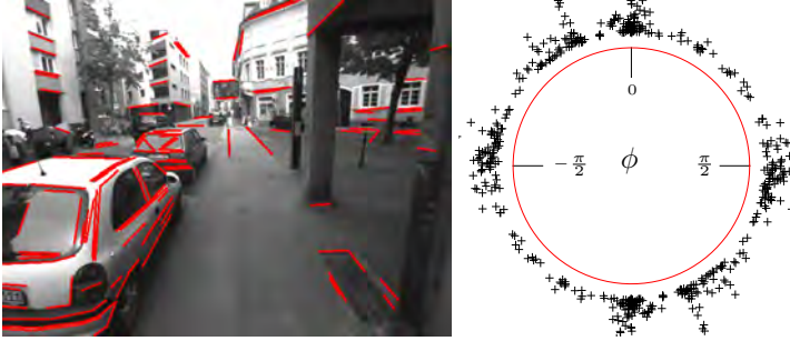
Figure 3.5: All hypotheses for horizontal vanishing directions obtained from the red edge segments. A zero azimuth angle \phi corresponds to the frontal direction and edge length is encoded with radius.
