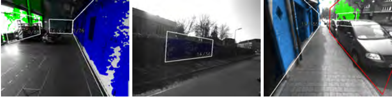
Figure 3.15: Examples of vertical structure modelled as planar surfaces. Right: During initialization new hypotheses are checked for plausibility. The red hypothesis is rejected, since it would occlude the green surface in the background.
