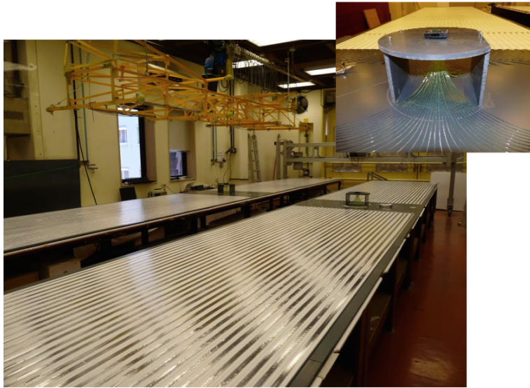
Figure 3.7: AMIGA module in the laboratory A module during production in the laboratory. The inset photo shows the fiber routing to the optical connector. Figure is taken from [70].
