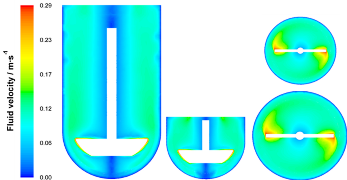
Fig. A.3 Fluid dynamic profile of an USP-2 apparatus with dimensions recommended by the FDA (left and right bottom) and with the dimensions recommended by Klein and Shah [20] (middle and right top) [19].
