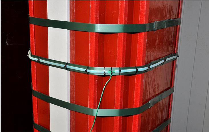
**Figure 5.5:** Pick-up coil around the limb of the transformer iron core. The coil is placed in the middle between the top and the bottom core yoke
