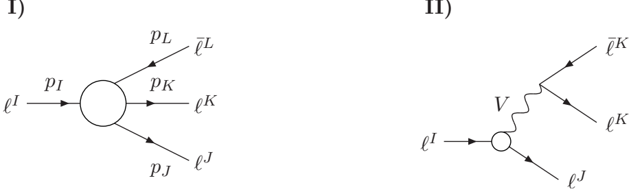
Figure 5. Diagrams contributing to \ell^I \rightarrow \ell^J \ell^K \bar{\ell}^L decay. I): 1PI irreducible box diagrams; II): penguin diagrams with V = Z, \gamma, h, H or A . For K = J crossed diagrams must be also included.
