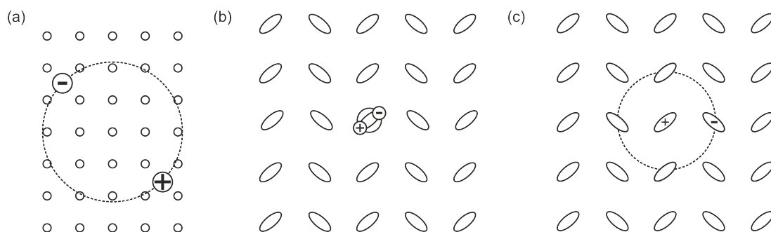
Figure 3.7: (a) In inorganic semiconductors, the binding energy of an excited Wannier exciton is so small that the thermal energy is large enough to dissociate it. The distance between the electron and the hole is much larger than the lattice constant. (b) Frenkel excitons are usually small-sized, and the electron and the hole are localized on the same molecule. (c) Charge transfer excitons can exist in molecular crystals, if the electron is promoted to an adjacent molecule, leaving one hole behind. Its size is between the size of Wannier and Frenkel excitons.[12]
