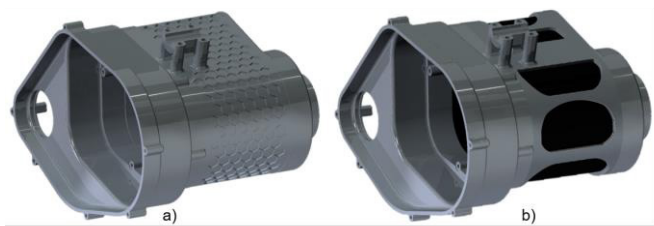
Fig. 7. Gearbox housing concepts a) with reinforcing honeycomb structure b) with sealing plastic cylinder
