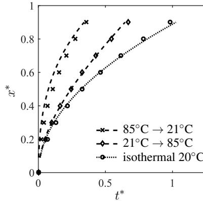
Figure 4.10.: Time function of non-isothermal flow with negative, positive, and zero temperature gradient  $dT/dx$  in channel with  $b_c = 40 \mu\text{m}$ ; experiments (markers) and model (lines); test piece temperature  $T_t(x)$  as displayed in figure 3.11a)
