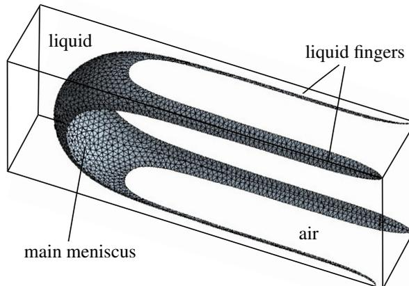
Figure 2.10.: Meniscus in a closed rectangular channel segment: Liquid-air interface with constant mean curvature computed with SURFACE EVOLVER [23] for a contact angle of  $5^\circ$
