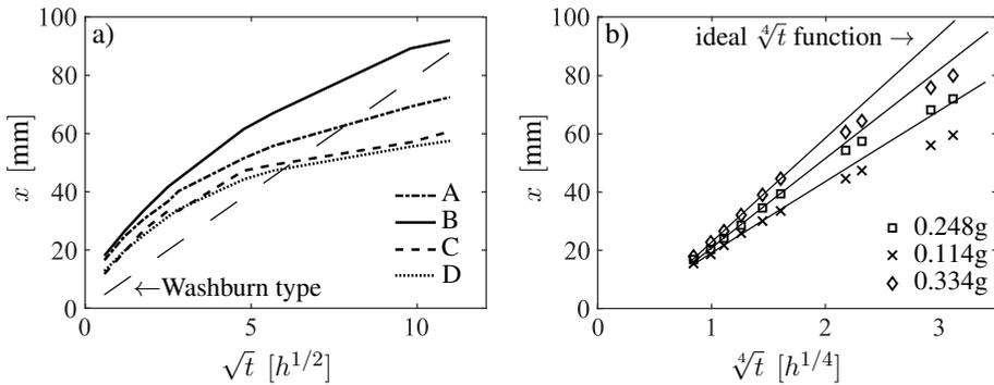
Figure 5.2.: Oil advancement dependent on a) four types of carrier paper A-D and b) on grease mass in grams (carrier filter paper grade 589/2, Whatman brand, GE Healthcare, USA)
