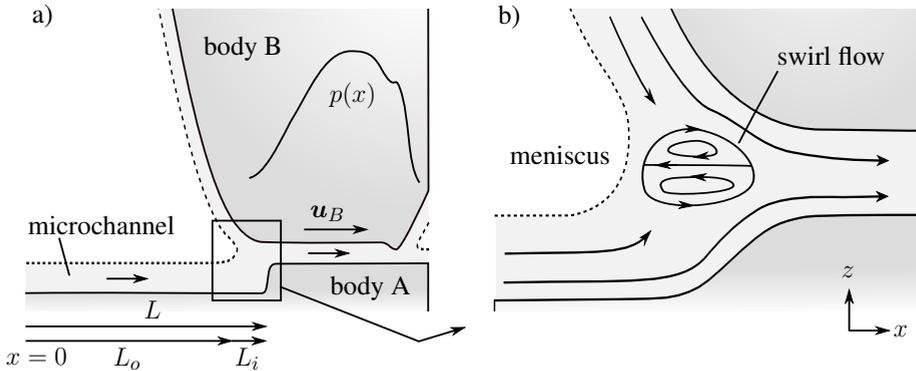
Figure 5.6.: a) EHL contact with characteristic pressure function, cf. [136, 196], adapted to include a supply microchannel; b) tribocontact inlet zone with capillary meniscus and developing swirl flow, adapted from [143]
