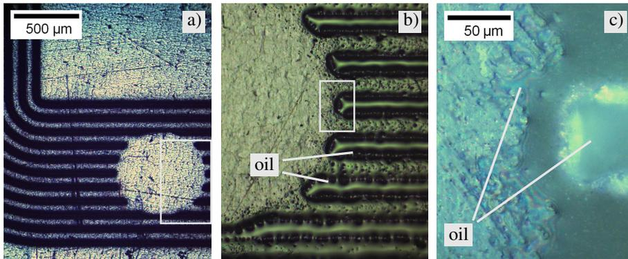
Figure 5.5.: Physics at the end of a microchannel (shown on the same type of test piece with from a) to c) increasing magnification, the white rectangles indicate the location shown in the next magnification step): a) overview of unfilled microchannels, with and without channel end; b) after filling the channels with oil, flow stops at the channel ends; c) surface roughness induced capillary forces pull small quantities of oil out of an ending microchannel
