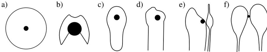
Figure 5.10.: Schematic representation of lubricant-filled area around the Hertzian ball-plate contact (in black) at different operating conditions: a) static case, b)-f) dynamic case based on interferometry and pressure measurements under different operating conditions in b) [143], c) [195] d) and e) [131] f) [160]
