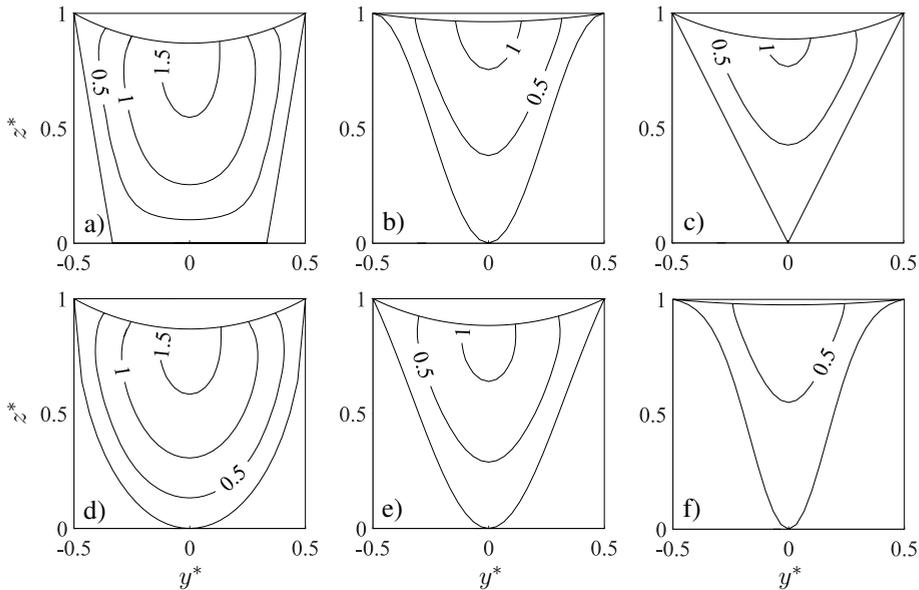
Figure 4.3.: Velocity profiles  $u^*(y^*, z^*)$  in different channel cross-sections: a) trapezoidal, b) sine, c) groove (v-shape), d) elliptical (u-shape), e) wide Gaussian ( $3\sigma$ ), f) narrow Gaussian ( $6\sigma$ ); for the rectangular cross-section see figure 4.5; comparison based on equal  $C$ , i.e., equal front meniscus pressure drop, channel length, and constant viscosity; for differences in upper meniscus see section 4.3
