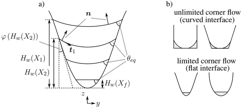
Figure 4.8.: Unlimited and limited corner flow depending on cross-sectional shape
