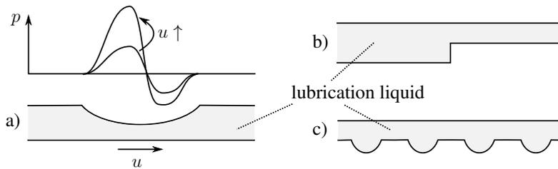
Figure 1.2.: Pressure generation within the tribocontact due to a) a protrusion, b) a step, c) dimples in the surface [66]
