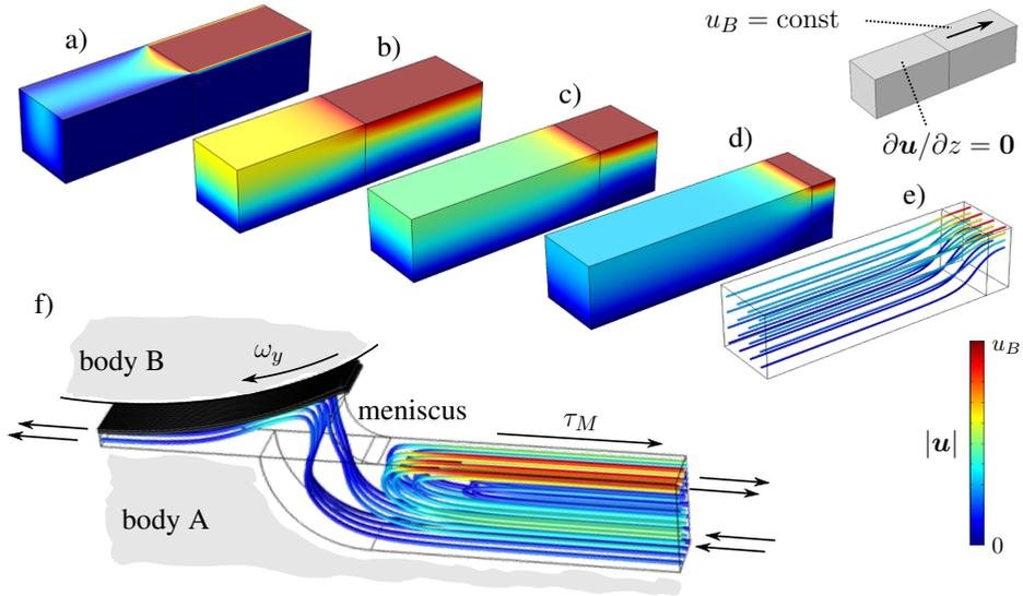
Figure 5.8.: Finite element computation of a Couette flow in a microchannel driven by the movement of a fraction of the channel's total upper surface: a) - e) pure channel flow, f) model of a tribocontact geometry including an influence of the Marangoni effect; see text for more details
