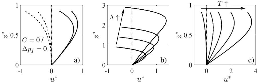
Figure 4.15.: Velocity profiles at  $y^* = 0$  (Gaussian channel) show that the consequences of the Marangoni effect can be influenced a) by the neglect of the capillary pressure (dashed lines) compared to the regular case (solid lines), b) by the aspect ratio, and c) by the absolute temperature; computation of b) based on Lenormand's formula for a rectangular channel (see text)
