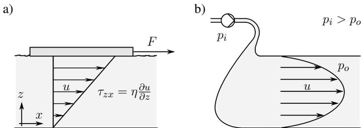
Figure 2.2.: a) Couette flow and b) Poiseuille flow with typical velocity profiles
