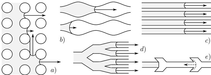
Figure 3.1.: Surface structures to transport liquids: a) pillars, b) converging-diverging channels, c) constant cross-section channels, d) tree-like structure, e) flow stopping geometry
