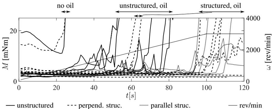
Figure 5.12.: Tribocontact failure of differently structured and lubricated test pieces; friction power is increased over time via rotational speed which causes a temperature rise; failure, if happening, is determined by a jump in moment
