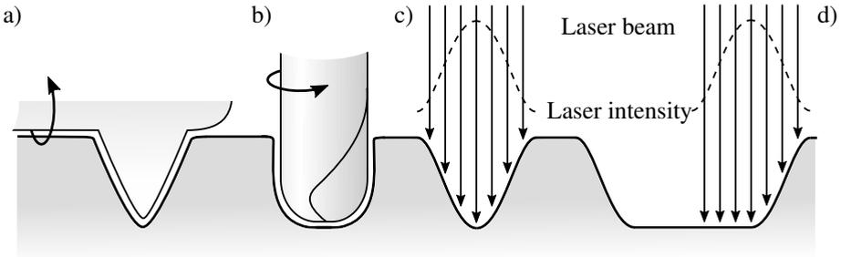
Figure 3.3.: Cross-sectional geometry of a microchannel as a consequence of fabrication (simplified illustration): a) b) micromilling, c) laser ablation d) laser ablation with multiple lines of operation
