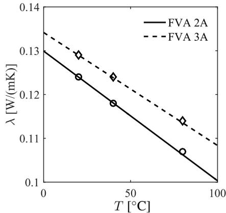
Figure 2.3.: Thermal conductivity of PAO reference oils FVA 2A (PAO ISO VG 32) and FVA 3A (PAO ISO VG 100) as a function of temperature; computation based on eq. (2.13) with measurement data from Bartel [9]
