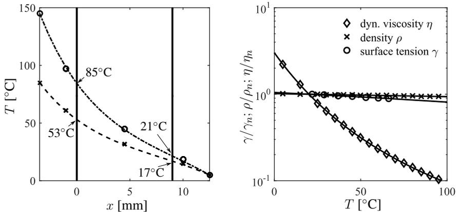
(a) Temperature distribution  $T_i(x)$  in POM test piece: measurement values (markers) and theoretical model (lines), cf. eq. (3.2); two variants which differ in hot side temperature (145°C vs. 85°C); the vertical lines indicate the flow domain for use in experiments, cf. figure 3.7
