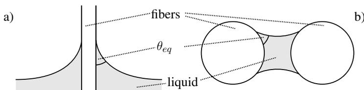
Figure 1.3.: a) Meniscus at a fiber immersed in a liquid with equilibrium contact angle  $\theta_{eq}$  [53]; b) liquid between two fibers [159]
