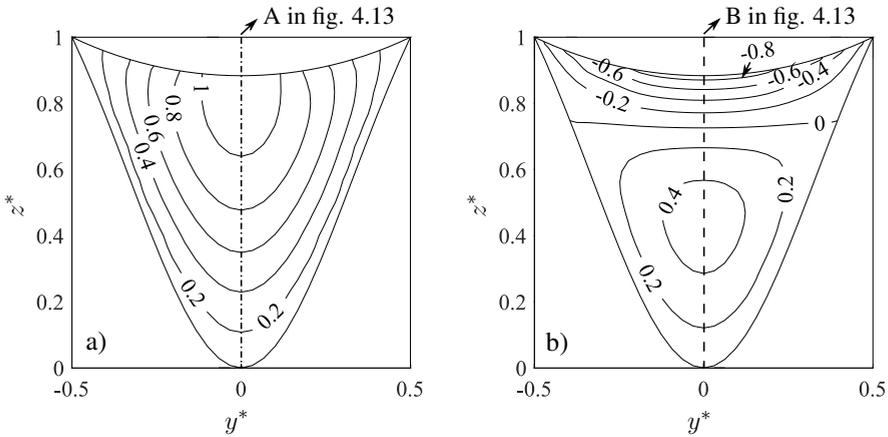
Figure 4.14.: Contour plot of the flow velocity  $u^*$ : a) base case of isothermal flow; b) the Marangoni effect pulls lubricant near the open surface away from the tribocontact which leads to simultaneous forward and backward flow in different fluid layers
