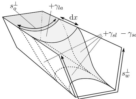
Figure 2.14.: Capillary force determination by free energy minimization approach
