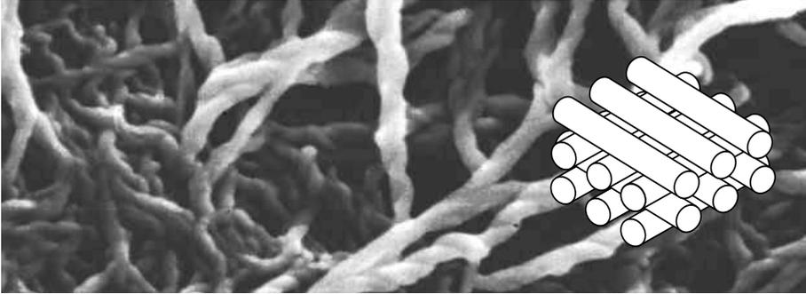
Figure 2.1.: SEM image and model of a grease: thickener structure, which serves as oil reservoir, is modeled in [5] as a stacked arrangement of fibers
