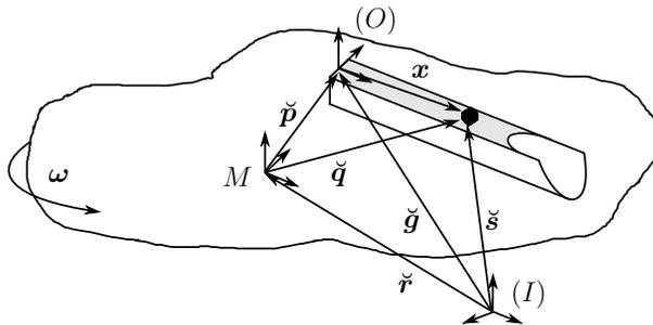
Figure 2.6.: Non-inertial channel frame of reference ( $O$ ), allowed to rotate and translate relative to the inertial frame ( $I$ );  $M$  is the origin of an auxiliary coordinate system in the non-inertial frame
