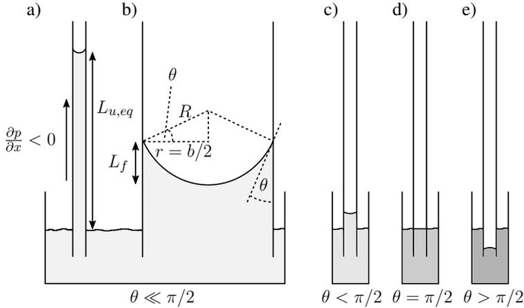
Figure 2.9.: Capillary rise in vertical circular tubes: Contact angle determines rise height
