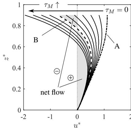
Figure 4.13.: Influence of the Marangoni effect on the flow rate: Velocity profiles in the channel center plane at  $y^* = 0$  under increasing Marangoni effect due to growing  $|dT/dx|$ : see figure 4.14 for the cross-sectional velocity field  $u^*(y, z)$  of cases A and B
