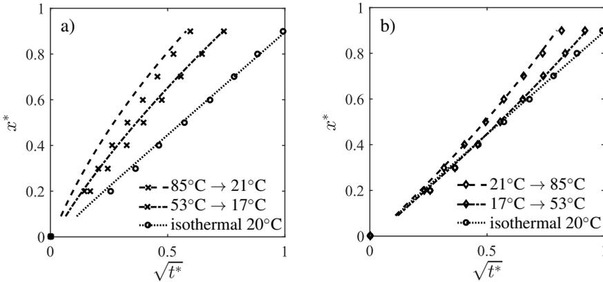
Figure 4.12.: Deviation from perfect Washburn behavior (isothermal case, straight line) of non-isothermal lubricant flow with negative (left) and positive (right) temperature gradient  $dT_i/dx$
