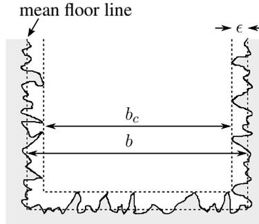
Figure 2.7.: Surface roughness in microchannels: Constricted diameter approach
