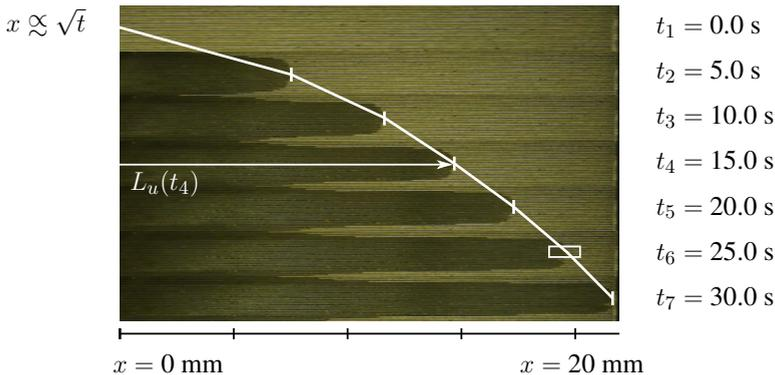
Figure 3.6.: Advancing oil front in multiple parallel channels; images taken at seven time points reveal Washburn-like behavior; the white rectangle indicates the location of figure 3.8 (taken in a different experiment); oil feed out of a brush (instead of using a reservoir) leads to a later start of the capillary flow at the sides of the main oil front
