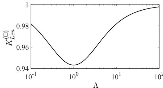
Figure 2.11.: Aspect ratio adjustment factor  $K_{Len}^{(\square)}$  from [128], computed with eq. (2.78)
