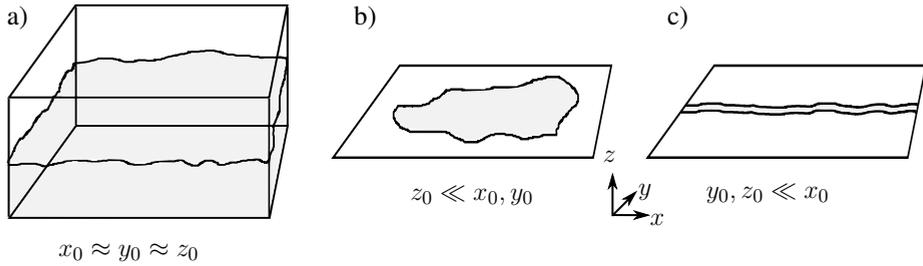
Figure 4.1.: Relation of characteristic length scales in a) bulk fluid, b) thin film, and c) microchannel
