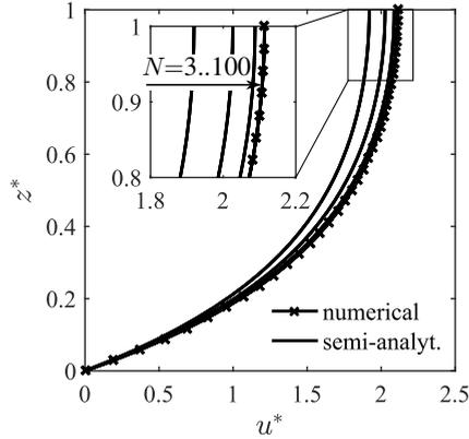
Figure 4.4.: Comparison of semi-analytical and numerical computation; the former based on sigma-approximated Fourier series, eq. (4.32), the latter being a finite differences approach, eq. (4.25) and (4.27)
