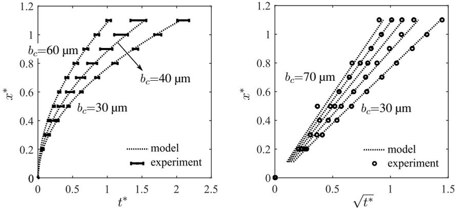
Figure 4.9.: Time function of capillary flow in open channels,  $\Lambda = 1$ ,  $b_c = 30 \dots 70 \mu\text{m}$ ; model fit (lines) via  $G_{ex}^{3\zeta} = 3.62$  to experimental data of channel with  $b_c = 60 \mu\text{m}$ ; experimental values of all channels are given with mean value (circles) or standard deviation (horizontal bars); same data as a function of  $t^*$  (left) and  $\sqrt{t^*}$  (right)
