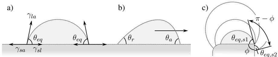
Figure 2.4.: Contact angles: a) equilibrium contact angle; b) advancing and receding contact angles; c) Gibbs criterion at sharp edges and analogous behavior at rounded edges
