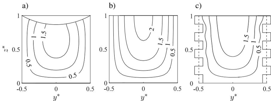
Figure 4.5.: Influence of changes in cross-sectional area on flow profile  $u^*(y^*, z^*)$ : a) by upper meniscus, c) by idealized surface roughness features in comparison to b) unrestricted flow area of open channel; absolute values comparable with figure 4.3
