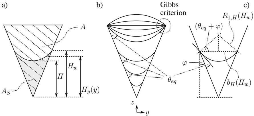
Figure 2.13.: Partially filled channel cross-section
