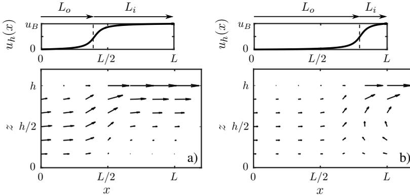
Figure 5.7.: Flow field  $\mathbf{u}(x, z)$  in the microchannel depending on the fractions of channel length inside ( $L_i$ ) and outside ( $L_o$ ) the tribocontact with upper surface velocity  $u_h(x)$ , which drives the flow, given above; no capillary contribution; computation based on the model given in the appendix; absolute flow rate  $q$  is higher in a)
