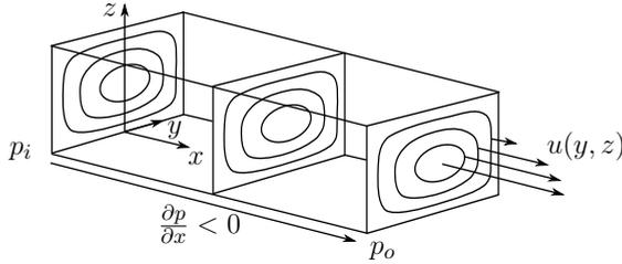
Figure 2.5.: Constant cross-section microchannel with pressure driven flow; contour lines of the velocity profile in cross-sections with maximum downstream velocity in the channel center
