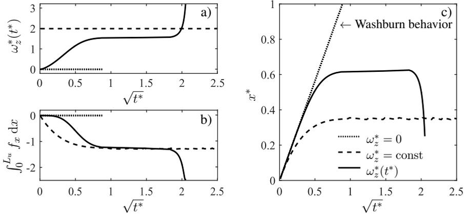
Figure 4.16.: Capillary channel flow in a rotating reference frame with flow direction radially towards the rotation axis (“spinning disk” case): no rotation (dotted line), constant angular velocity (dashed line) and varying angular velocity (solid line) as specified in a)
