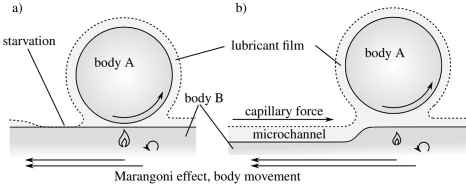
Figure 1.1.: Tribocontact a) in starvation and b) with capillary lubricant supply by a microchannel; thermal effects (heat is generated in the tribocontact) and body movement may draw the lubricant away from the tribocontact with the capillary effect as a countermeasure
