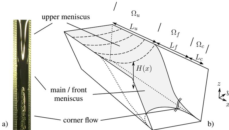
Figure 4.7.: Liquid-air surface in an open channel with a) square and b) trapezoidal cross-section; conceptual split-up into three regions: upper meniscus region  $\Omega_u$ , front meniscus region  $\Omega_f$ , and corner flow region  $\Omega_c$ ; picture a) has approximative character only as taken in the static case against gravity in a channel with  $b = h = 1000 \mu\text{m}$
