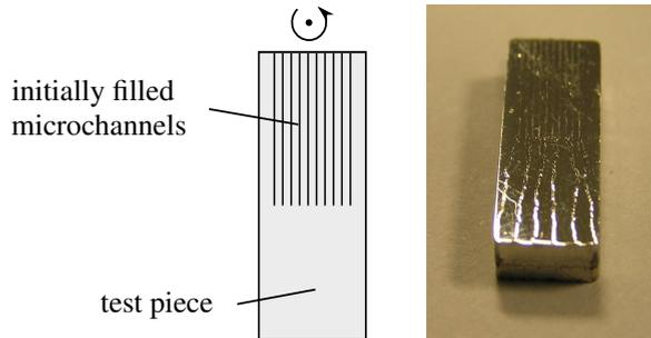
Figure 5.4.: Structured microchannels end at half length of the test piece; channels are initially filled with oil as seen in figure 5.3b); subsequent centrifugation as described in [29] leads to oil flow out of the channels (right image)
