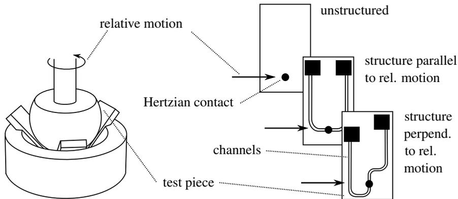
Figure 5.11.: Basic experimental setup to test capillary supply effectiveness of a tribocontact; experiments were conducted with three different sets of test pieces with  $b_c = 50 \mu\text{m}$ ,  $\Lambda \approx 1$  and further dimensions similar to figure 3.7
