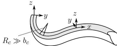
Figure 4.6.: Slight channel curvature based on eq. (4.36) allows the use of curvilinear coordinates
