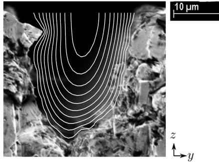
Figure 4.2.: Overlay of cross-sectional velocity profile  $u(y, z)$  (contour lines shown) and SEM image of channel lasered into stainless steel with undesired irregular boundary
