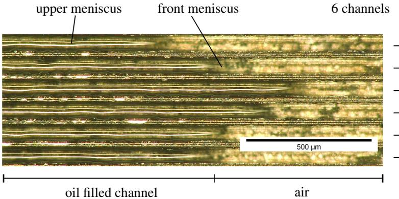
Figure 3.8.: Oil front in six parallel microchannels; microscope focal plane at the upper channel edge with the channel bottom blurred; light reflections give insight into the shape of the menisci
