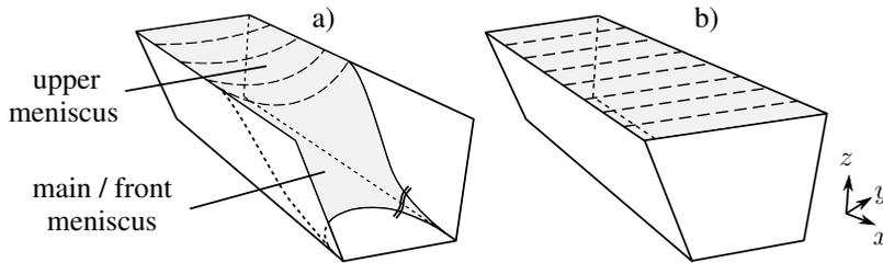
Figure 5.3.: Channel end effect: a) Capillary flow having not yet reached channel end (same as figure 4.7); b) breakdown of capillary flow with vanishing menisci at channel end
