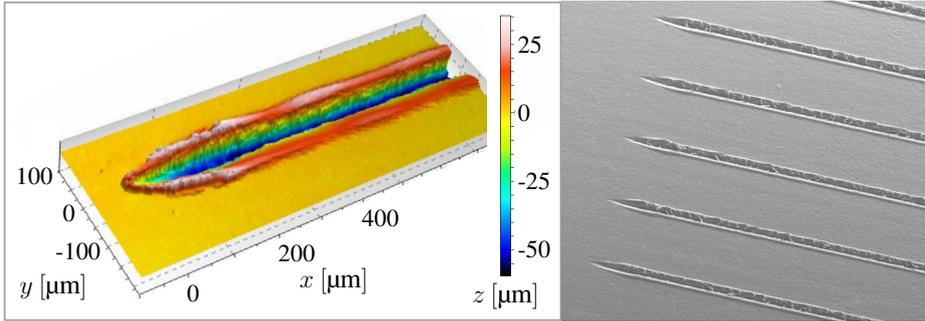
Figure 3.5.: Microchannels of approximately triangular cross-section fabricated by peripheral milling into polyamide 6-6; SEM image (right); geometry measurement (left) via confocal microscopy (M. Egner, Bosch)
