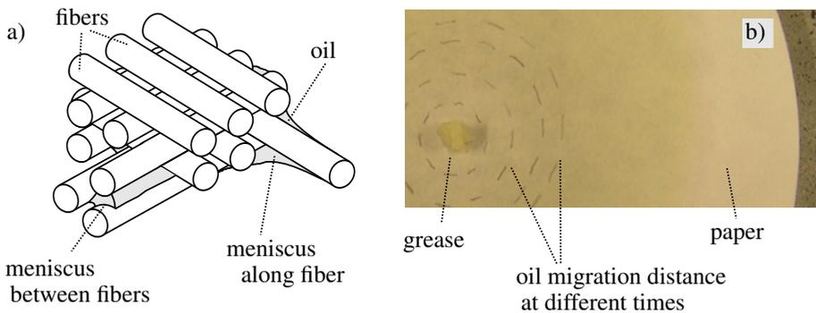
Figure 5.1.: a) Expected capillary effects within a grease if the thickener structure is modeled as proposed by [5]; b) interplay of two capillary systems: grease and carrier structure (pictured is the quantitative ashless cellulose filter paper grade 589/2, Whatman brand, GE Healthcare, USA)
