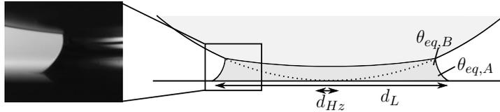
Figure 5.9.: Fluid-filled domain around the static ball - plate contact
