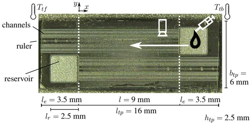
Figure 3.7.: Test piece with a total of 24 straight microchannels
