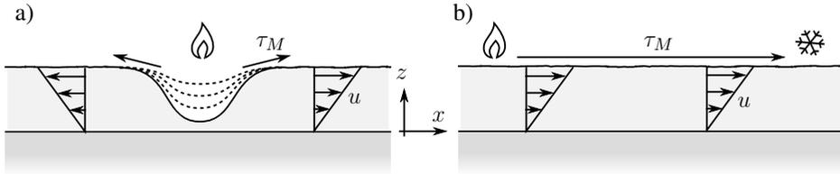
Figure 2.8.: Thermal Marangoni effect: a) local heating leads to thinning of fluid film as liquid flows away; b) temperature gradient leads to Couette flow away from hot region towards cold region
