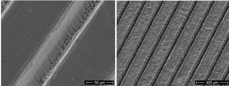
Figure 3.4.: Microchannels fabricated by femtosecond laser ablation into a) stainless steel, b) polyoxymethylene (POM), source: H. Besser / M. Mangang (KIT IAM)
