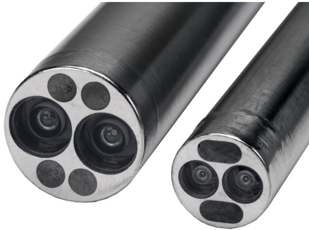
Figure 2.4: The stereo endoscope of the da Vinci surgical system. ©2017 Intuitive Surgical, Inc.
