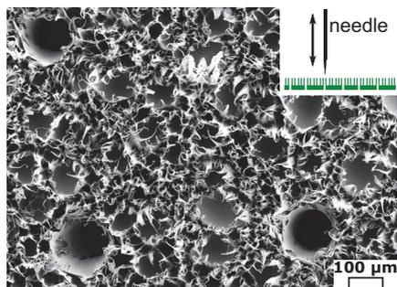
**Figure 3.7:** Microneedle perforated nanofur. SEM image of thin nanofur film perforated with a microneedle with diameter  $100\ \mu\text{m}$ .
