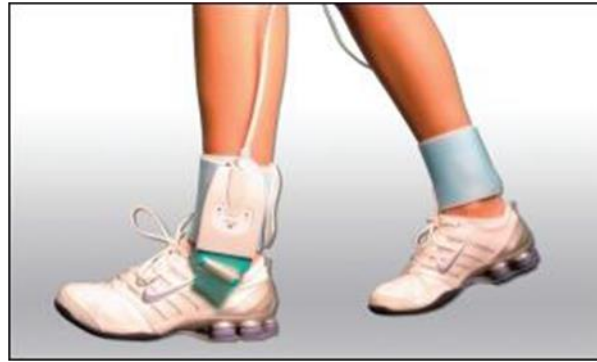
Figure 4-8. In-shoe plantar pressure analysis system [121]
