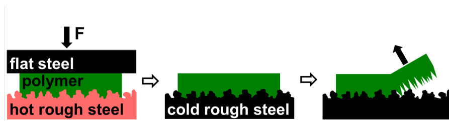
Figure 4.14: Cold pulling fabrication process. A polymer foil is pressed into a sandblasted steel plate by hot embossing. After cooling down the mold and opening the tool, the polymer foil is manually pulled from the rough mold surface, which results in elongation of the polymer and the formation of nanohairs.
