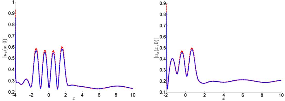
Fig. 2. Amplitudes of vertical displacements on the surface of a steel isotropic layer (the Poisson ratio  $\nu = 1/3$ ) containing a crack under the excitation by a vertical point source: (a)  $\bar{\omega} = 0.97$ ,  $a = 1.49$ ,  $h = 0.4$ ,  $x_0 = 4$ ; (b)  $\bar{\omega} = 1.57$ ,  $a = 1$ ,  $h = 0.4$ ,  $x_0 = 2$ .
