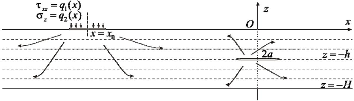
Fig. 1. Multilayered structure with a crack
