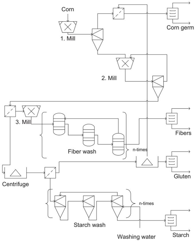
Figure 5.4: Scheme of the corn wet milling process
