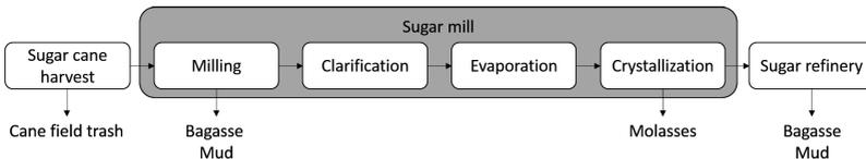
Figure 5.5: Scheme of the sugar cane processing (Meyer [227])
