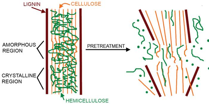
Figure 2.3: Breakdown of lignocellulosic complex (Mosier [239])
