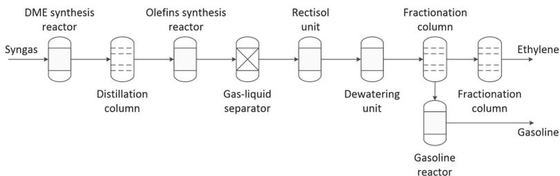
Figure 5.10: Process flow sheet for the production of ethylene f. syngas (Trippe et al. [149])
