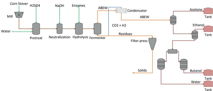
Figure 5.7: Process flow sheet for the production of ABE from corn stover
