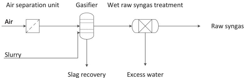
Figure 5.9: Process flow sheet for the production of syngas from slurry (Trippe et al. [357])
