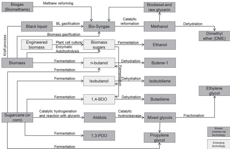
Figure 2.6: Emerging routes to bio-based alcohols (Nexant [260])
