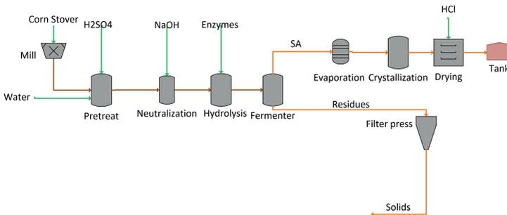
Figure 5.8: Process flow sheet for the production of succinic acid from corn stover
