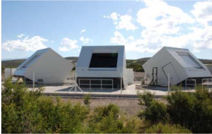
Figure 2.7 High Elevation Auger Telescopes (HEAT) photograph. This three new telescopes are deployed close to Coihueco to complement its field of view, allowing the detection of lower energy showers.
