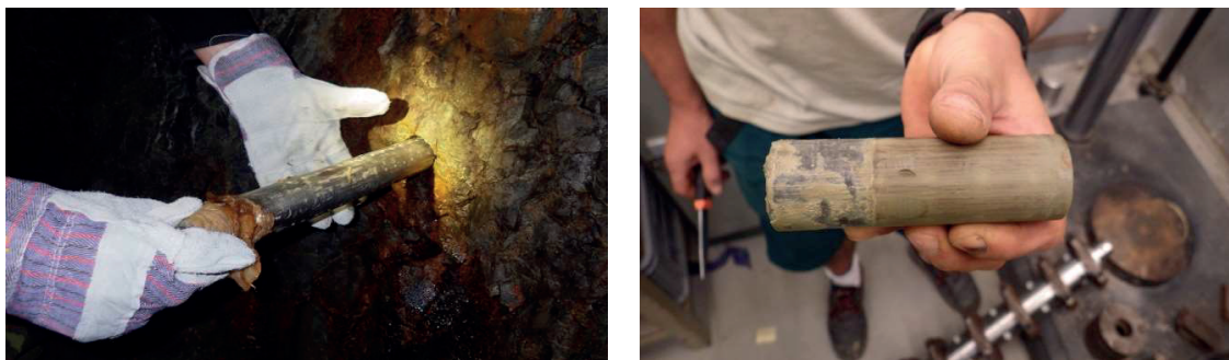
Figure 1: Extraction of the cartridge from the borehole (left) and cement / bentonite sample squeezed out from the cartridge (right).
