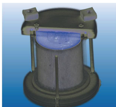
Figure 2: \mu CT-image of the sample with cut at the injection port. The joint between salt and cement, as well as the head space, are detectable, but below image resolution of 30 \mu m.
