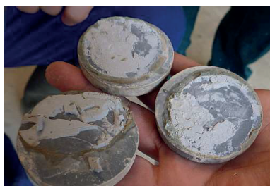
Figure 4: Formation of new phases (white areas) on the boundary of hardened cement with bentonite (Vessel 4) after 9 months of interaction.
