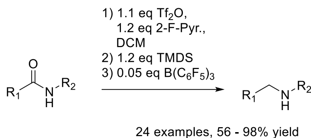
Scheme 14: One-pot catalytic reduction of amides to secondary amines using TMDS as reducing agent. \text{Tf}_2\text{O} = triflic anhydride, 2-F-Pyr. = 2-fluoropyridine, \text{B}(\text{C}_6\text{F}_5)_3 = tris(pentafluorophenyl)boron.
