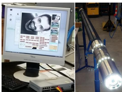
Fig. 4: GeoKam prototype test, in the geothermal test-hall at the IAI.
