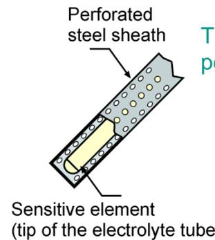
Tip of oxygen sensor with perforated steel sheath.
