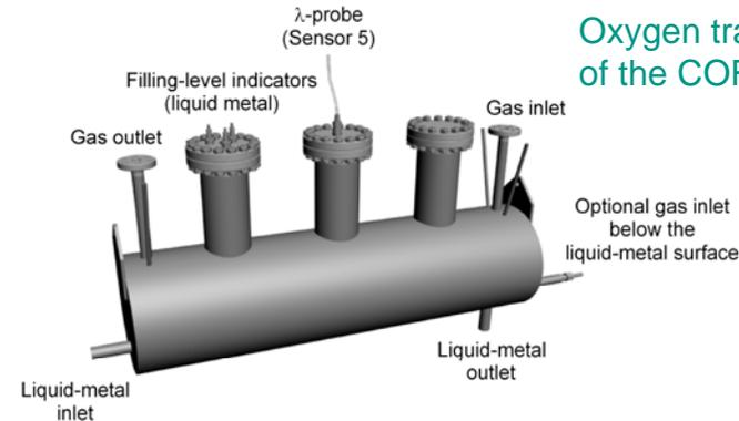
Oxygen transfer device of the CORRIDA loop.
