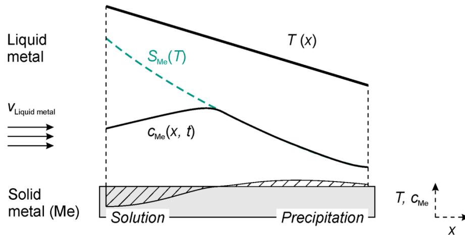
Solution and re-precipitation of solid metal determined by the temperature-dependent solubility  $S_{Me}$ .
