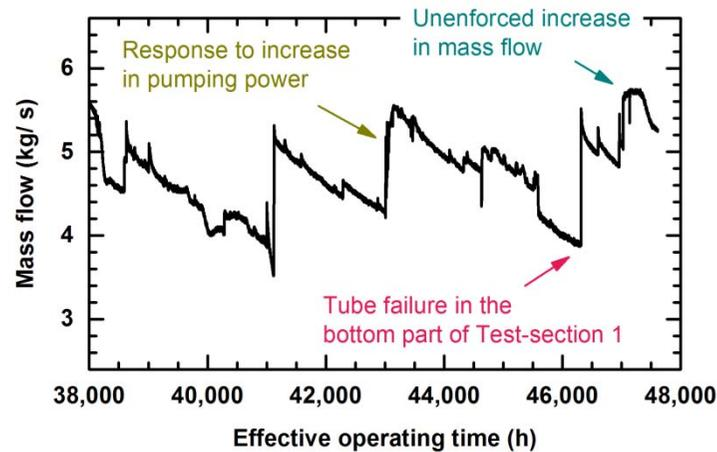
Mass flow during stage of partial plugging.
