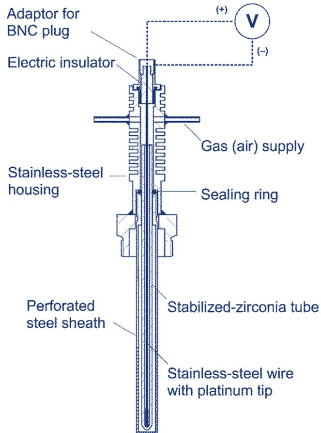
Design of oxygen sensors installed to the CORRIDA loop.
