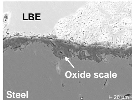
Sample T6, close to the site of tube failure after 66,000 h.
