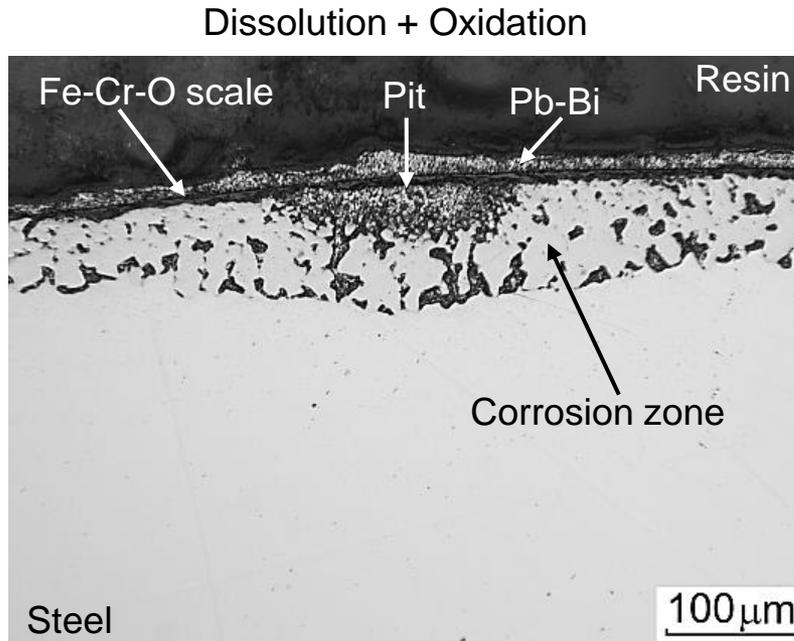
Corrosion zone Fe-Cr-O scale
