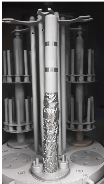
Figure 6.5: Rotating platform of the magnetron sputtering facility at IAM-AWP with one BASE-Nb-Steel coated sample. A foil covers the areas not to be coated during the sputtering process (Nb transition tube, stainless steel tube and some parts of the ceramic).
