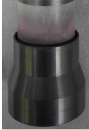
Figure 6.3: Change in the color of the BASE in the area close to the brazing.
