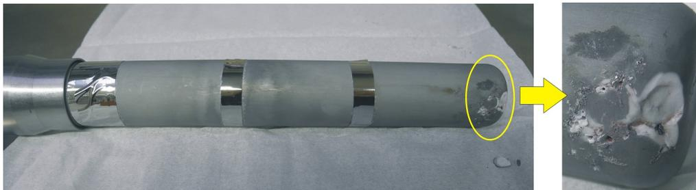
Figure 6.6: Ceramic coated with continued d.c. magnetron sputtering. During the sputtering process a large plasma concentration appeared in the ceramic dome that damaged it.
