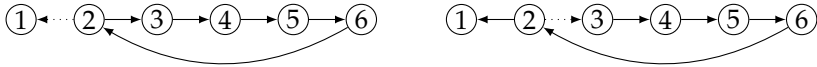
(a) With C = \{(1, 2)\} , we need one permutation and one copy operation. (b) With C = \{(2, 3)\} , we need two permutation operations and one copy.
