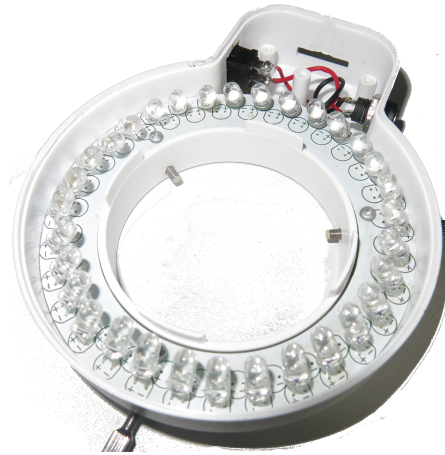
Figure 3.3: Close-up of the IR LED ring that was retrofitted to the Nikon microscope to allow for permanent illumination during a PMR experiment.
